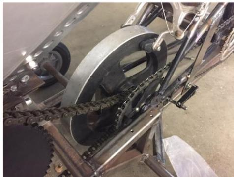
**Figure 3.** Assembled drivetrain.
