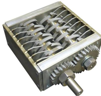
**Figure 2.** Filamaker shredder.
