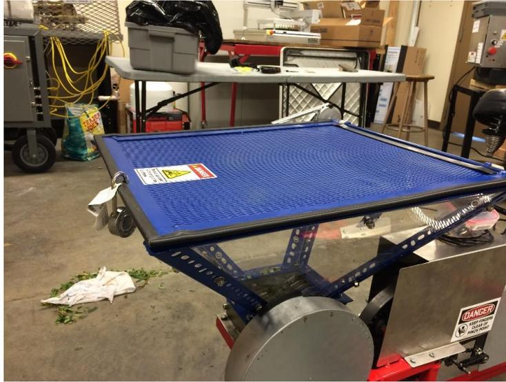
**Figure 4.** Hopper and sheet metal safety mechanisms.
