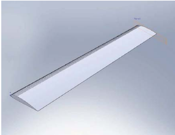
Figure 1: Model of a twisted, variable chord proof of concept blade.
