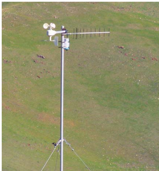
Figure 4: Wind measurement unit with long range (10 km) radio link
