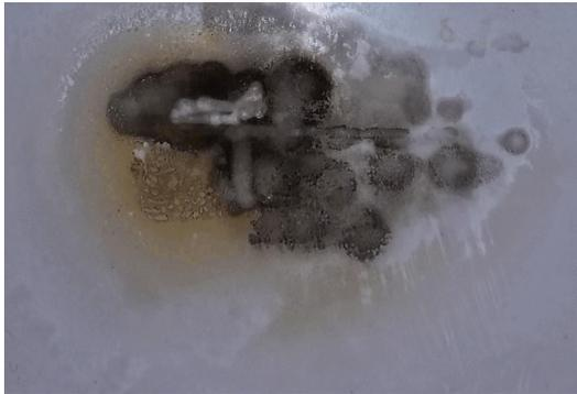
**Figure 12.** Laboratory experiment **quartz blast shield** that has undergone multiple ablation measurements. The ring of brown debris shows basalt sample ejecta from recent measurement. The black shows ejecta from the multiple laser ablation measurements embedded in the quartz.
