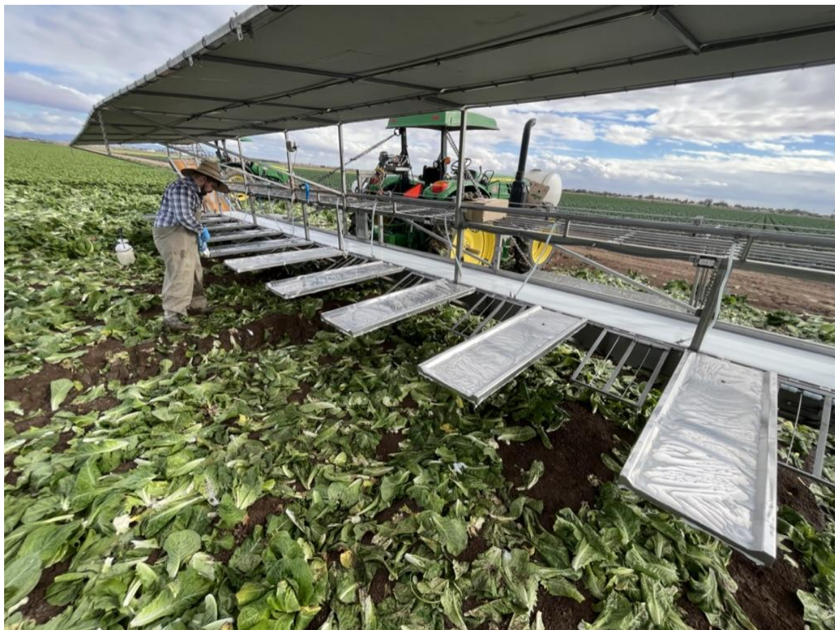
Figure 2. Harvester from an agricultural food processing site in Santa Maria, California. The coupons utilized in the efficacy test serve to simulate the harvester conveyor belt and trays that compose this piece of agricultural machinery.
