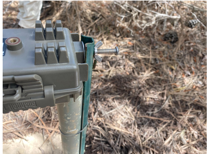
Figure 2. Image of the DP2 Station C1 set-up. Note that the sand was manually transferred to the station in order to cover up pine needles, which the AI could potentially detect as a tail.
