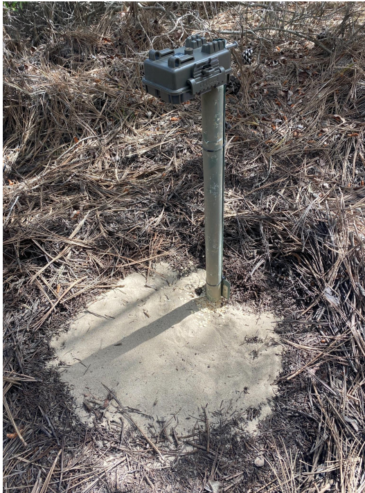
Figure 2. Image of the DP2 Station C1 set-up. Note that the sand was manually transferred to the station in order to cover up pine needles, which the AI could potentially detect as a tail.
