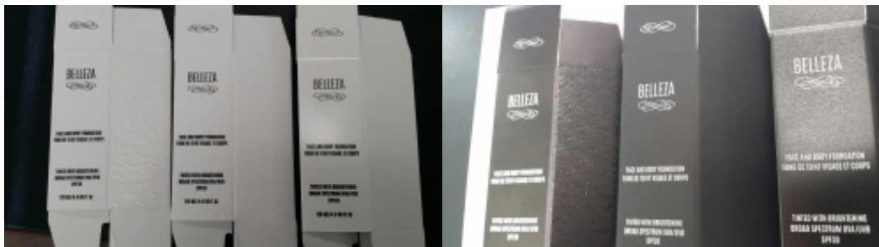
Figure 1 - Photos of fictitious packages in white and black designs with Hi Rise (left), Soft Touch (middle) and no coating.
