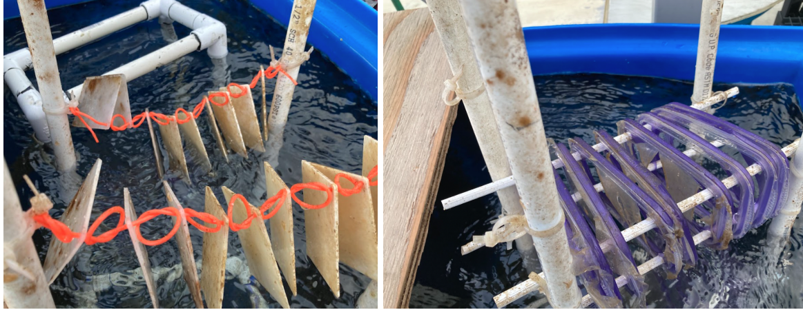
Figure 2. Experimental layout for submersion of plastic formulations in flow-through seawater. Chip submersion is shown on the left and film submersion shown on the right.
