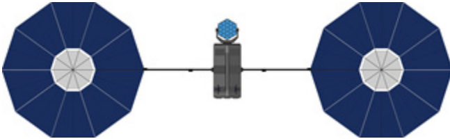
Figure 3. Conceptual design of the deployed spacecraft with two 15 m PV arrays that produce 50 kW each at the beginning of life for a total of 100 kW electrical, ion engines at the back, and the laser array pointed directly at the viewer. A 2 m diameter laser phased array is shown with 19 elements, each of which is 1-3 kW optical output. From Kosmo et al. [13].
