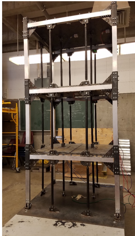
Figure 2: Shake Table Model
