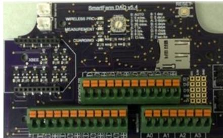
Figure 2. Wireless soil moisture sensor data acquisition board
