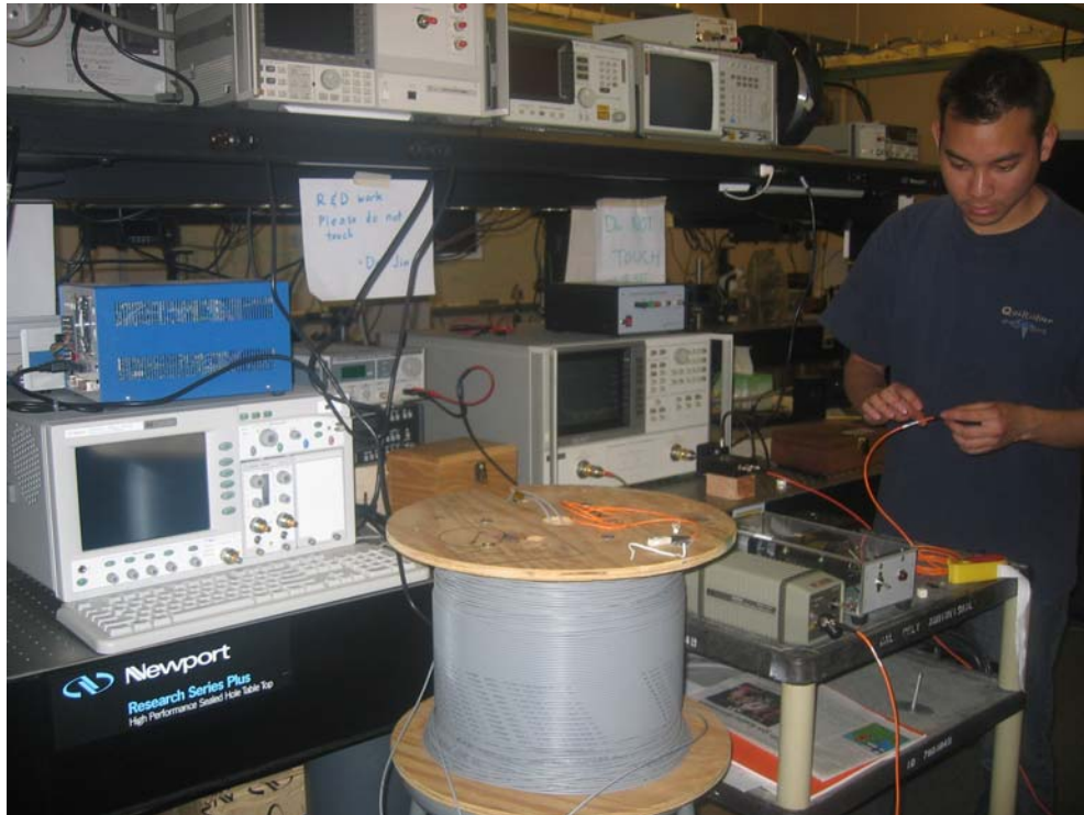
Figure 4. James De Leon standing by his master thesis setup of multimode fiber characterization for an industrial partner.
