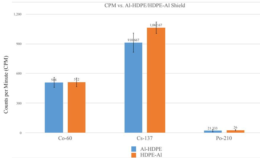
Figure 4: CPM ( $\pm$  S.E.) comparison between Al-HDPE and HDPE-Al shield orientations for Co-60, Cs-137 and Po-210. Only Cs-137 produced a difference ( $p < 0.05$ ) in shield effectiveness based on orientation.
