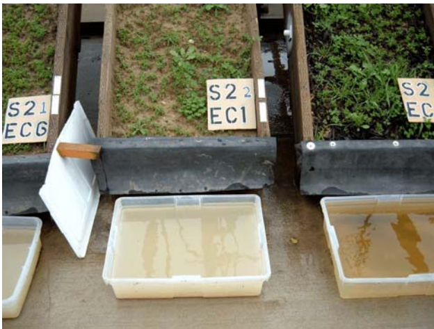
Figure 8. Sandy clay loam (S2) control (EC1) high sediment.
