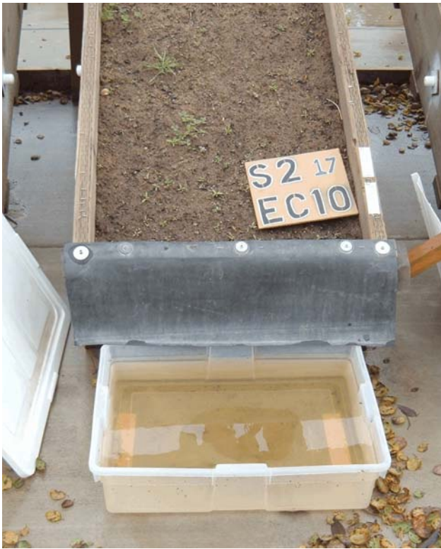
Figure 9. Sandy clay loam (S2) with 16 mm hydroseed (EC 10): low sediment.
