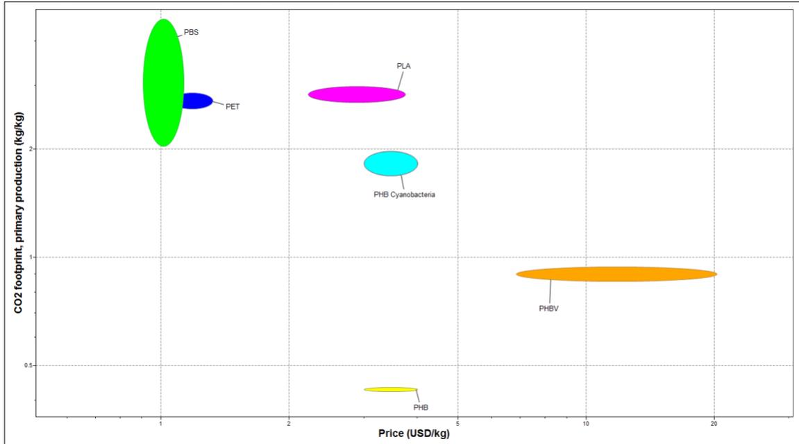
Figure 3. Price and CO2 Footprint of polymers PLA, PBS, PHB, PHBV, PHB Cyanobacteria, and PET. PLA and PLA were sourced from Granta Edupack. PHB, PBS, PHBV and PHB Cyanobacteria were all input from the data in Appendix B.
