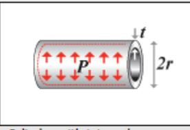
**Cylinder with internal pressure**
