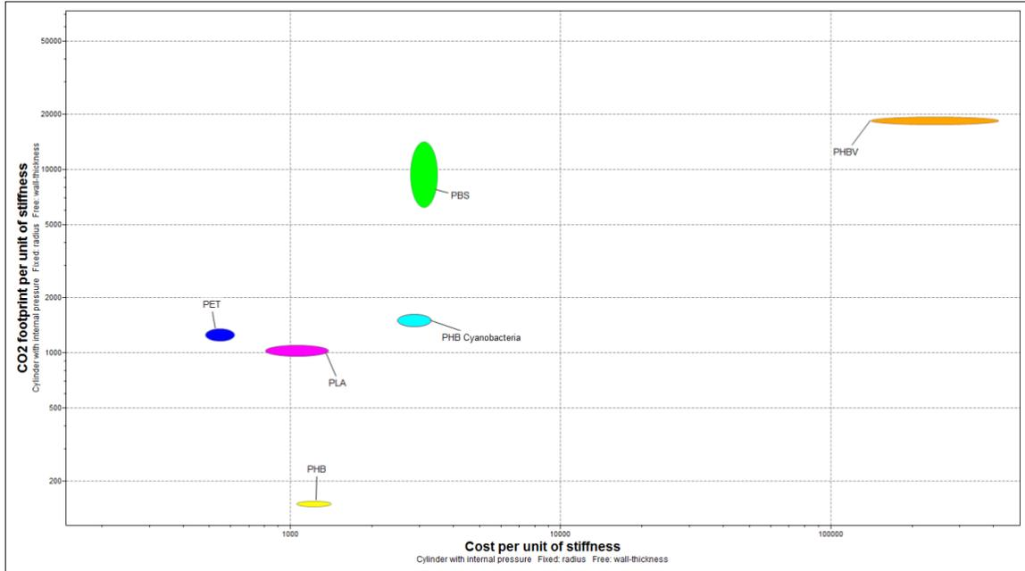
Figure 6. Carbon footprint and price of 1 water bottle per unit of stiffness.
