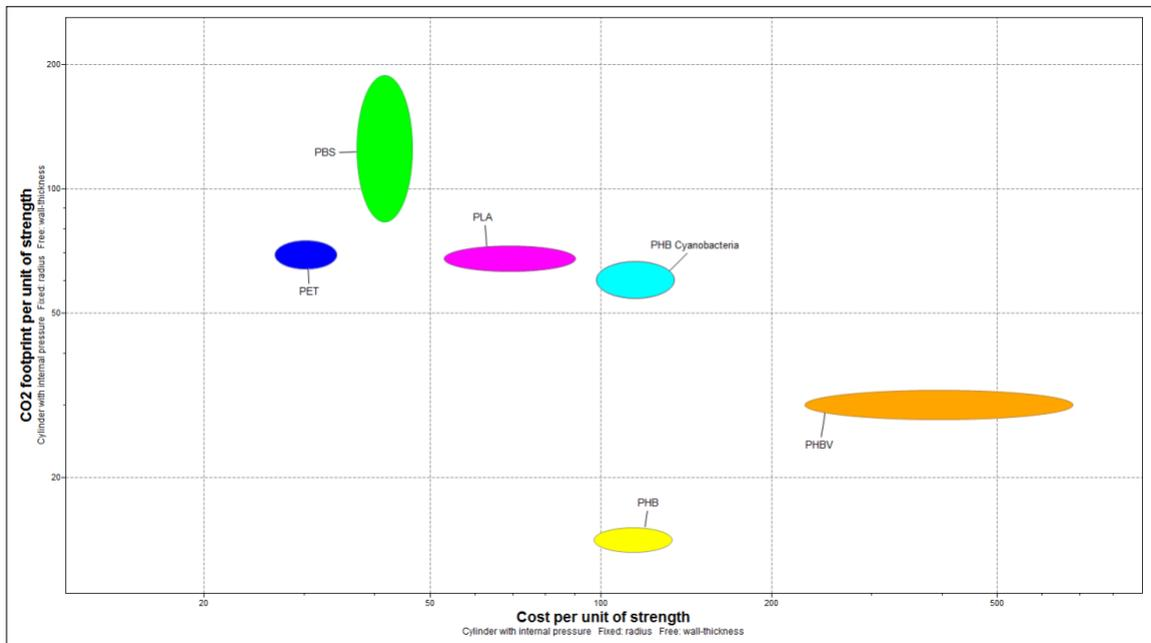
Figure 5. Carbon Footprint and price for 1 water bottle per unit of Strength.
