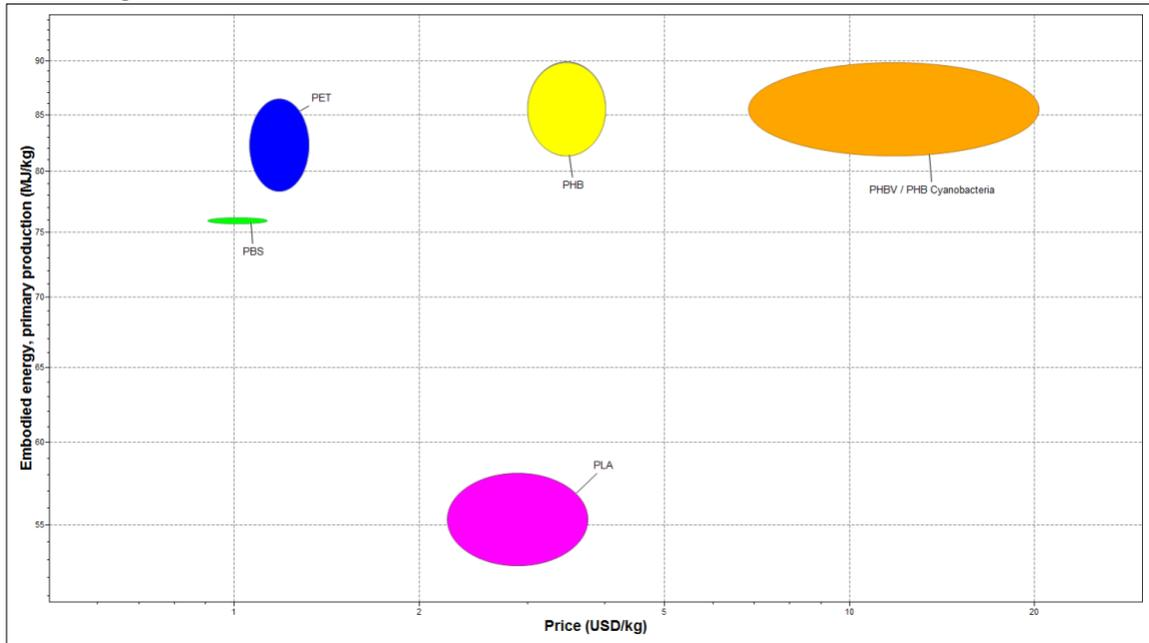
Figure 4. Price and Embodied Energy of polymers PLA, PBS, PHB, PHBV, PHB Cyanobacteria, and PET. PLA and PLA were sourced from Granta Edupack. PHB, PBS, PHBV and PHB Cyanobacteria were all input from the data in Appendix B.
