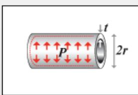
**Cylinder with internal pressure**
