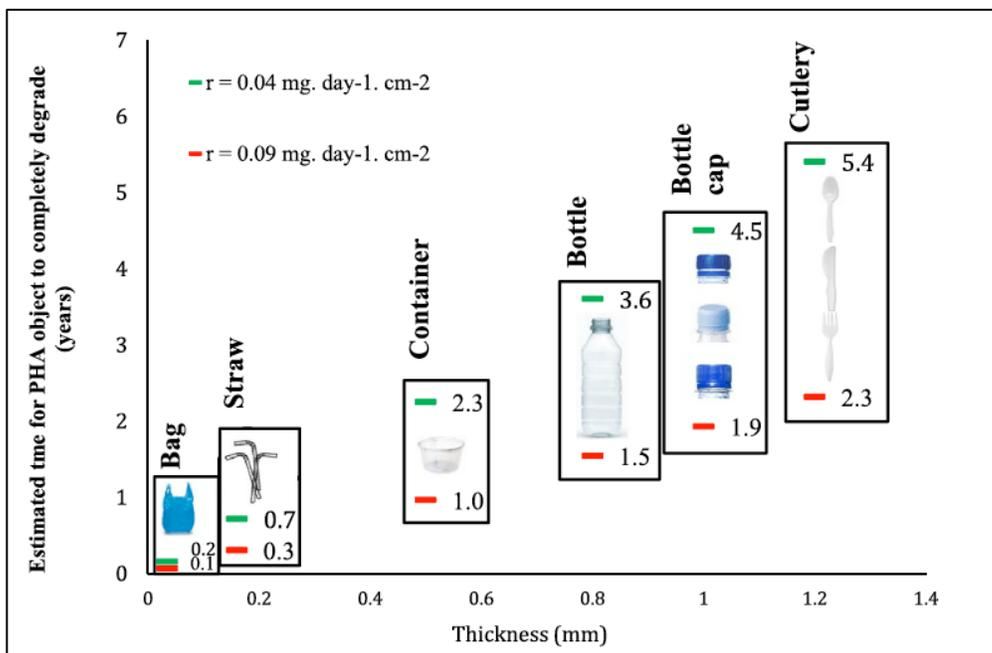
Figure 2. PHA degradation. Lifetime values estimated using the 95% confidence interval for the mean of the rate of biodegradation of PHA in the marine environment. Figure sourced from Dilkes-Hoffman et al., 2019.
