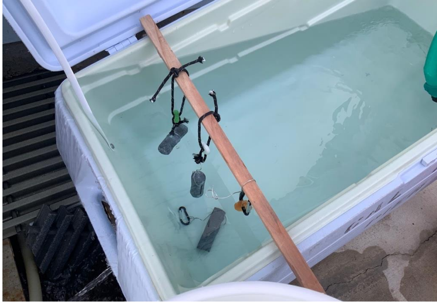
Figure 16: Flowing water testing apparatus. 3 tests occurring at the same time, bottom most has ended and broken already
