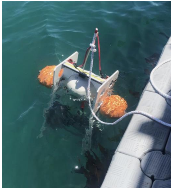
Figure I10: The Final Buoyancy test conducted for the Lander with all Parts of the Finished Prototype on Board.
