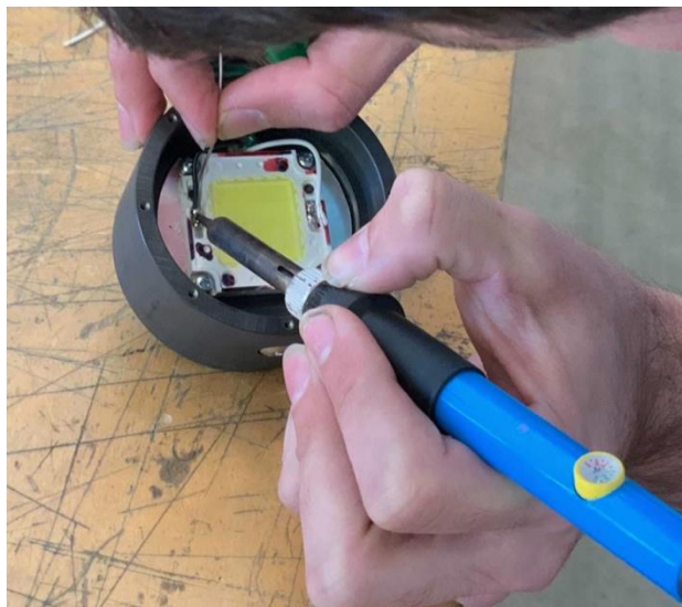
Figure 42: Soldering LED Leads for the Light before Filling the Housing with Oil
