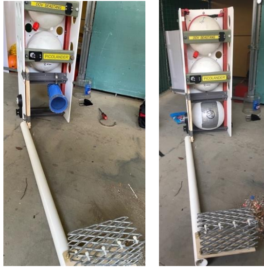
Figure 15: Single camera setup to view deep sea animals attracted to the bait.
