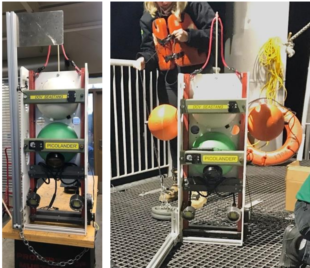
Figure 28: Finished Lander with and without Buoyancy Spheres
