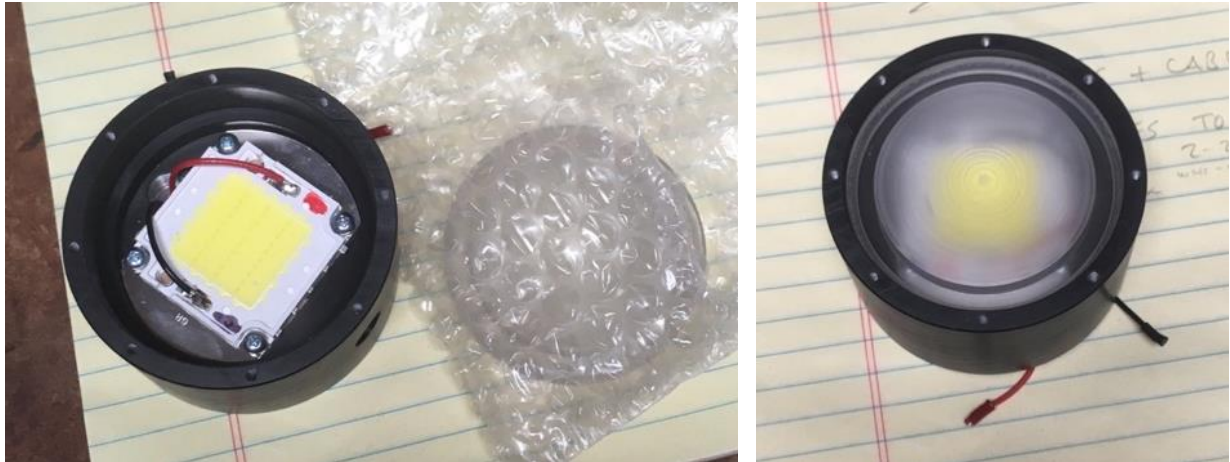
Figure 18: LED Light With and Without Diffuser
