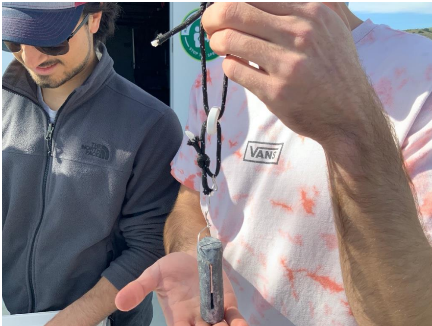
Figure I3: LifeSavers (middle, white) attached to weight (bottom) with open loop (top) for attaching apparatus to dowel rod.
