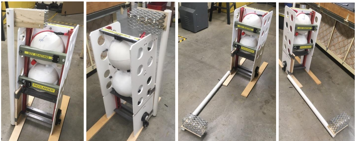
Figure 13: Full Scale Prototype of Single Drop Arm with Bait Cage
