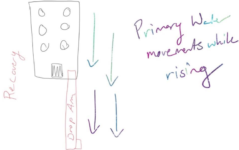
Figure 12: Sketch of Lander with Single Drop Arm Bait System in Ascent (Side View)
