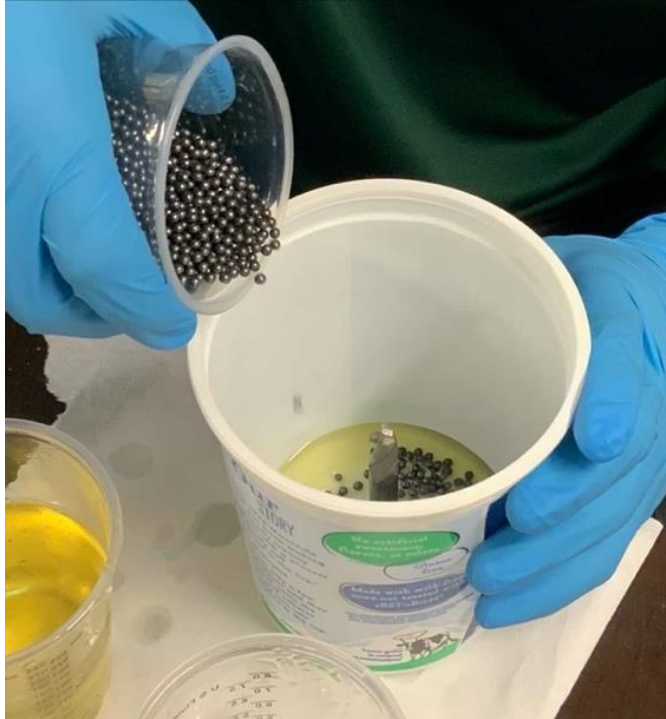
Figure 44: Making counterweights from lead shot and epoxy/urethane
