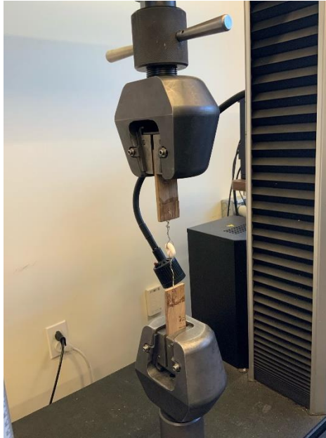
Figure I1: Instron Tensile Test setup with LifeSavers attached
