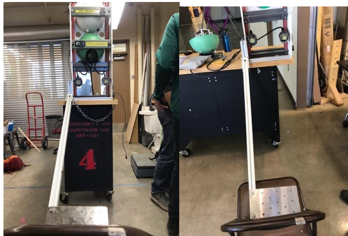
Figure 18: Testing the angle of the bait arm relative to the camera
