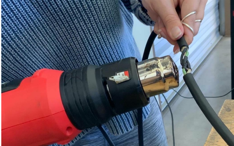
Figure 43: Heating the Shrink Tubing for the CamDo and Light System
