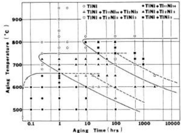
Figure 5. TTT diagram describing aging behavior for Ti-52Ni<sup>4</sup>.
