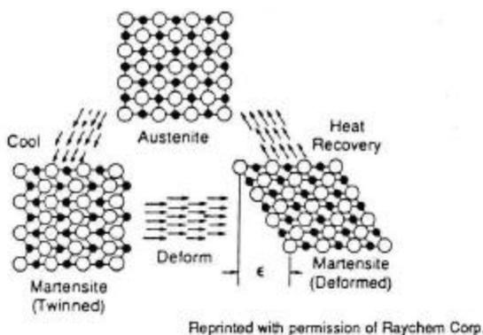
Figure 1. Phase changes associated with the shape memory effect<sup>1</sup>.
