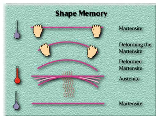
Figure 2. Demonstration of the shape memory effect<sup>2</sup>.
