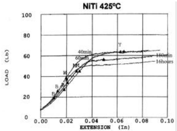
Figure 9. Tensile test results for NiTi heat-treated at  $425^{\circ}\text{C}$  for four different times. Longer anneal times produce lower plateau stresses for the martensitic transformation due to higher  $A_f$  temperatures (that are closer to room temperature).
