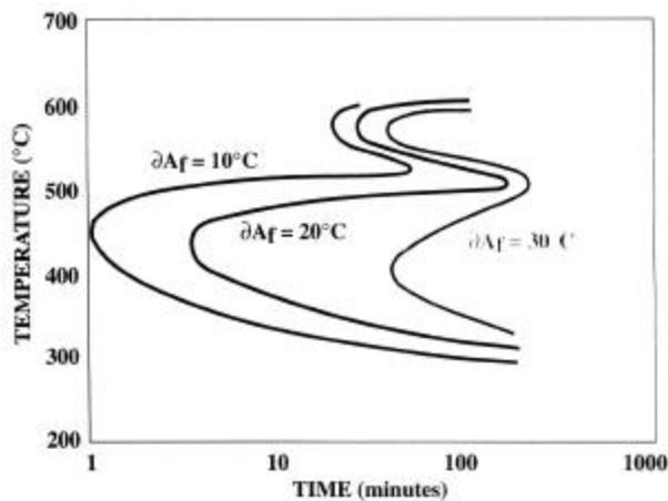
Figure 8. Contour curves of changes in the  $A_f$  temperature of NiTi upon annealing at specific temperatures and times<sup>6</sup>.
