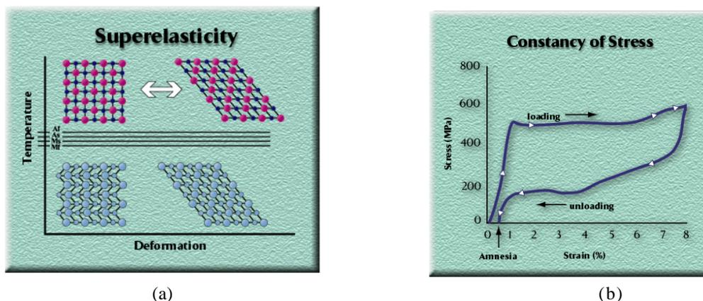
Figure 3. a) Superelasticity involves the stress-induced phase transformation of austenite to martensite. b) The plateau stress is associated with the martensitic transformation<sup>2</sup>.
