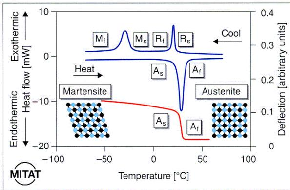
**Figure 6.** Differential scanning calorimetry and free recovery of the same processed wire. Note that upon cooling the wire transforms to R-phase prior to the martensitic transformation. Upon heating, both techniques provide similar  $A_s$  and  $A_f$  temperatures as the (monoclinic) martensite transforms to the (cubic) austenite.<sup>5</sup>
