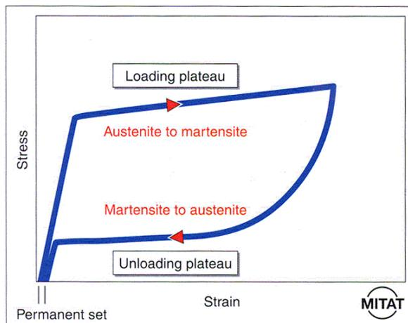
**Figure 7.** Schematic stress-strain curve of superelastic Nitinol. There is a transformation from austenite to martensite that begins at the apparent yield stress. The plateau stress remains nearly constant with increasing strain as the amount of martensite increases. Upon unloading, the martensite reverts to austenite along the unloading plateau. The 'permanent set' measures any residual strain.<sup>5</sup>
