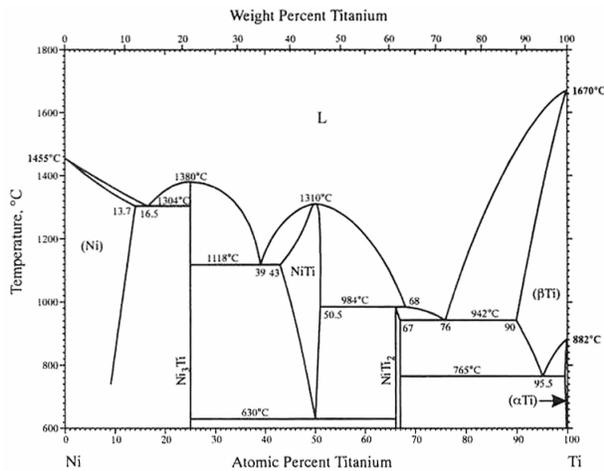
Figure 4. The Ni-Ti phase diagram<sup>3</sup>.
