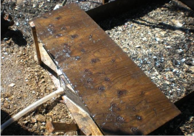
**Photo 1:** Plot with protective top to prevent water from directly entering catchment area.
