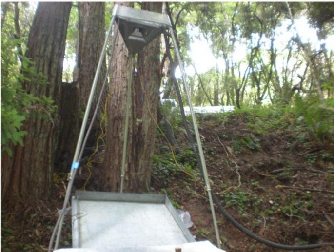
**Photo 2:** Calibration sheet covering plot.
