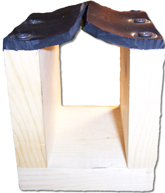
Figure 12. Soft rubber flap prototype created for testing.
