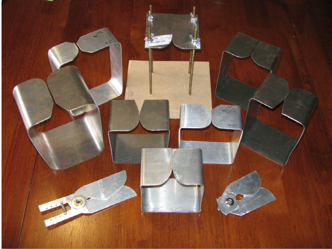
Figure 17. Chip removal device prototypes used to determine final design
