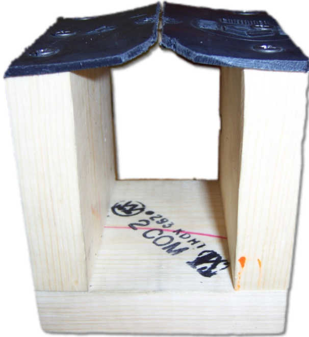
Figure 13. Firm rubber flap prototype created for testing.
