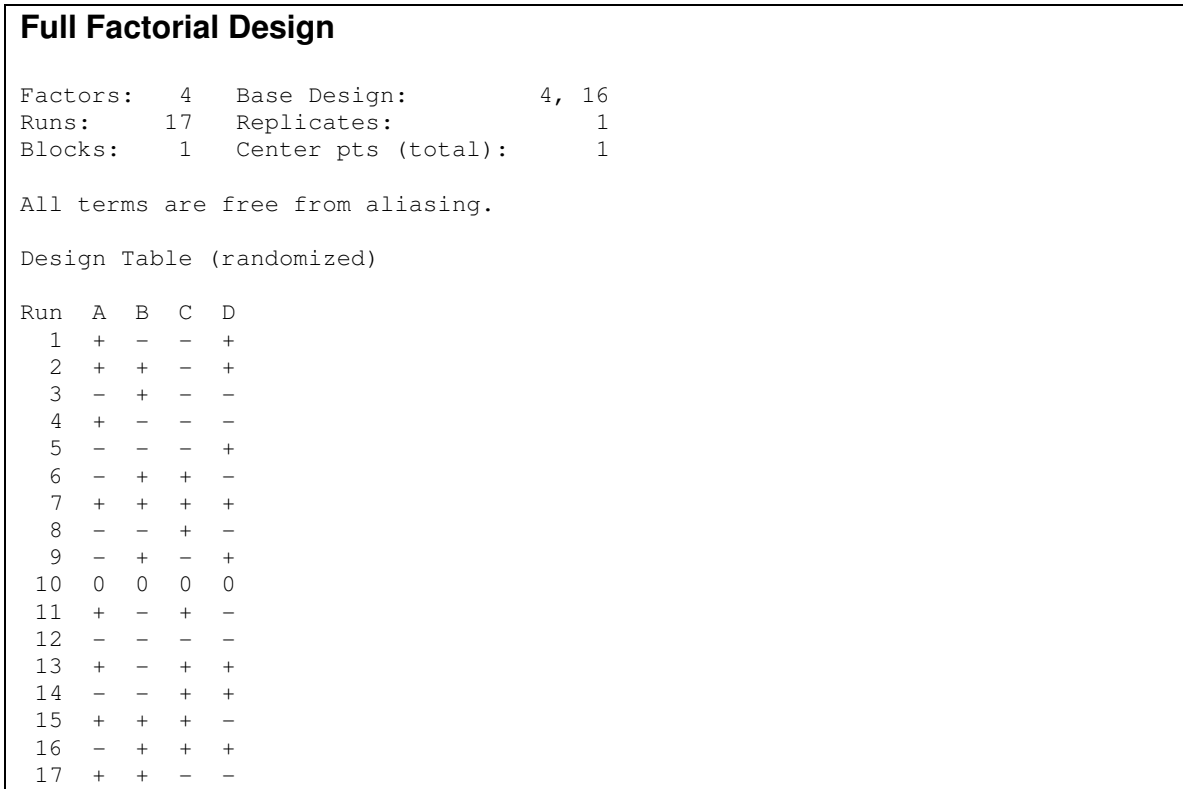
Figure 1: Minitab Output for DOE (+) = upper level treatment (-) = lower level treatment (0) = midpoint between treatment levels
