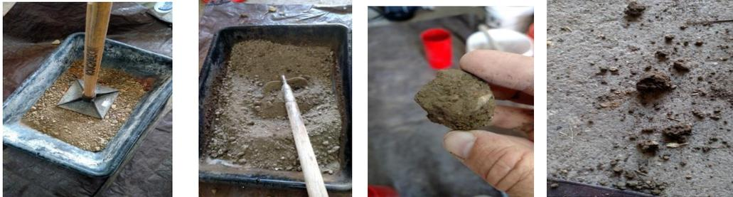
Figure 5(Left): 8”x8” steel tamper used to crush up soil
