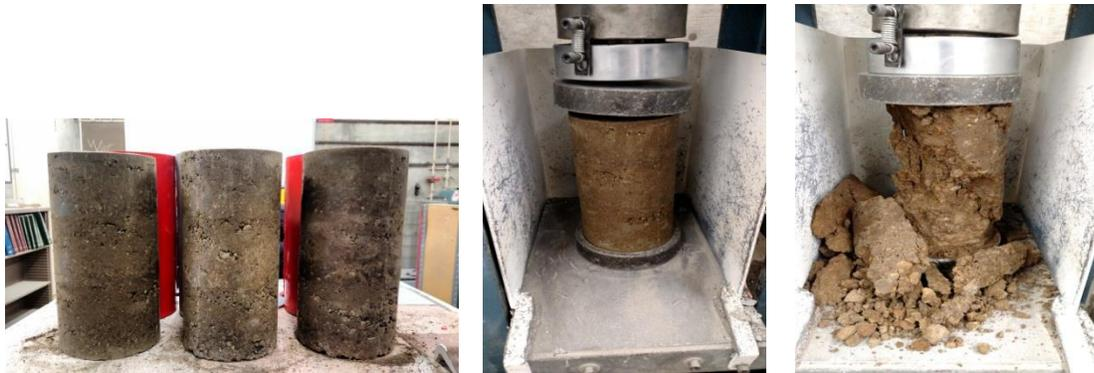
Figure 10 (Left): Rammed earth samples that were just taken out of the molds. Notice the dark color of the soil, these samples could still use some curing time to get their full strength potential.
