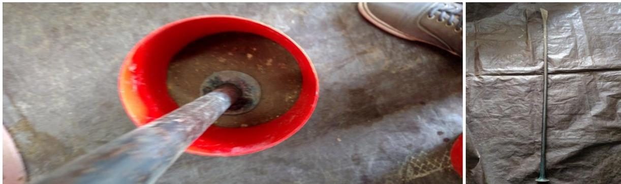
Figure 8(Left): First layer being compacted into a test cylinder.
