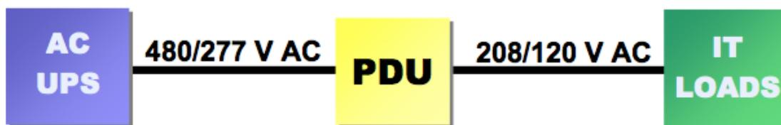
**Figure 4: Common AC Distribution in North America**
