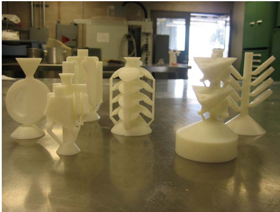
Figure 1 – Sprue patterns generated by rapid prototyping in ABS material
