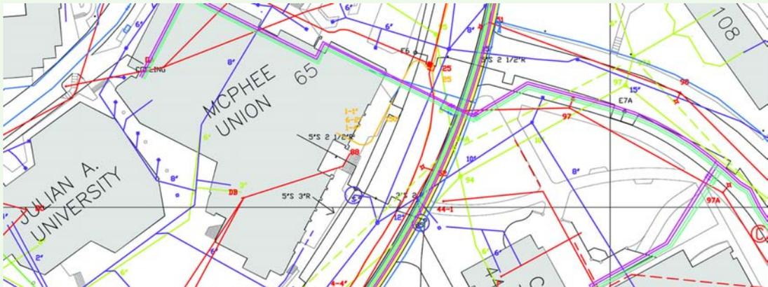
Current computer database, Atlas B. Atlas B shows it all, useful for digging and avoiding unpleasant surprises. Here the colors are simplified. Blue indicates water. Purple indicates storm drains. Cyan indicates chilled water.
