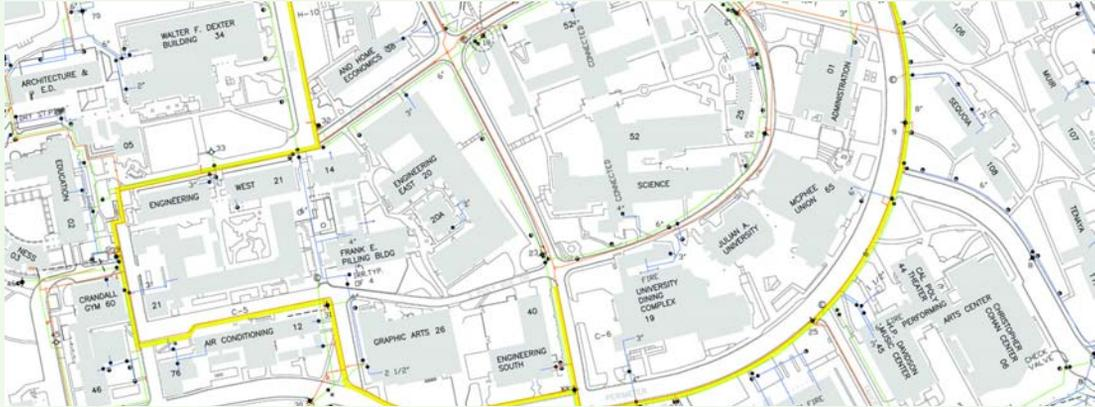
Current computer database, Atlas A. Atlas A shows utility systems one-at-a-time. This detail shows water with the colors representing different water systems and pressure zones.
