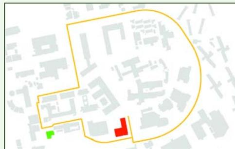
The Old Power House is shown in green; in red is the building that houses Cal Poly’s heating and cooling plant #4 (Engineering South, #40). The Utilidor, a mile-long vault under sidewalks that delivers hot water, chilled water, and drinking water, is shown in orange.
