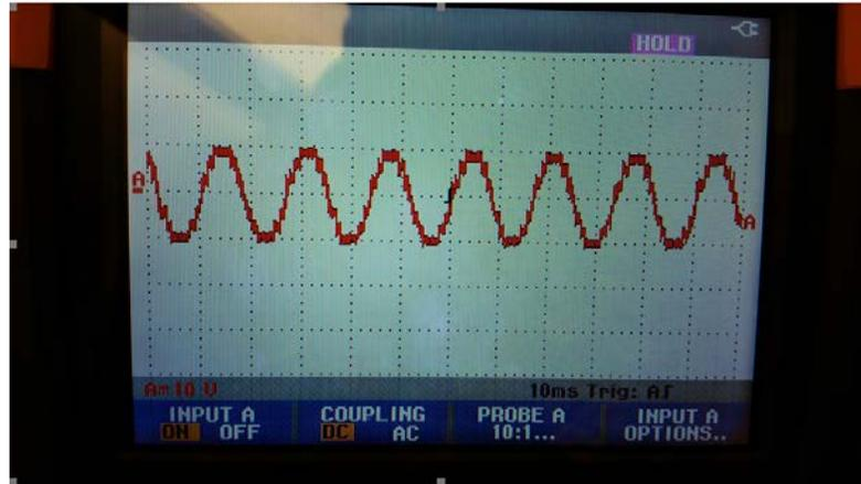
Figure 11. Final Inverter Output
