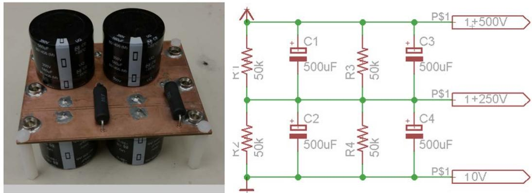
Figure 7. Input Capacitor Stage
