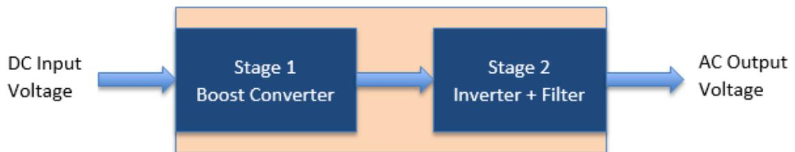
Figure 1. High Density Inverter – Level 0 Block Diagram
