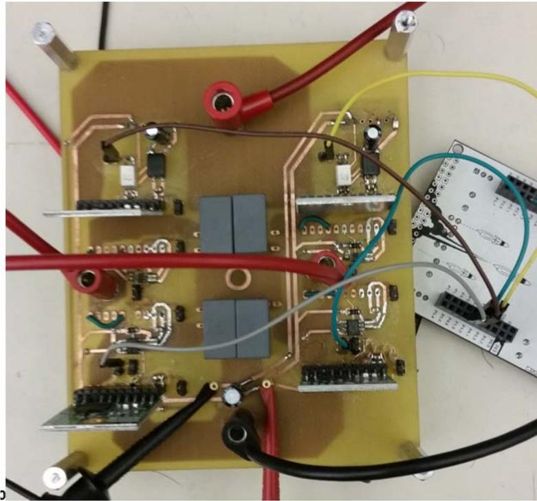
Figure 9. Final Revision of the Power Inverter Stage
