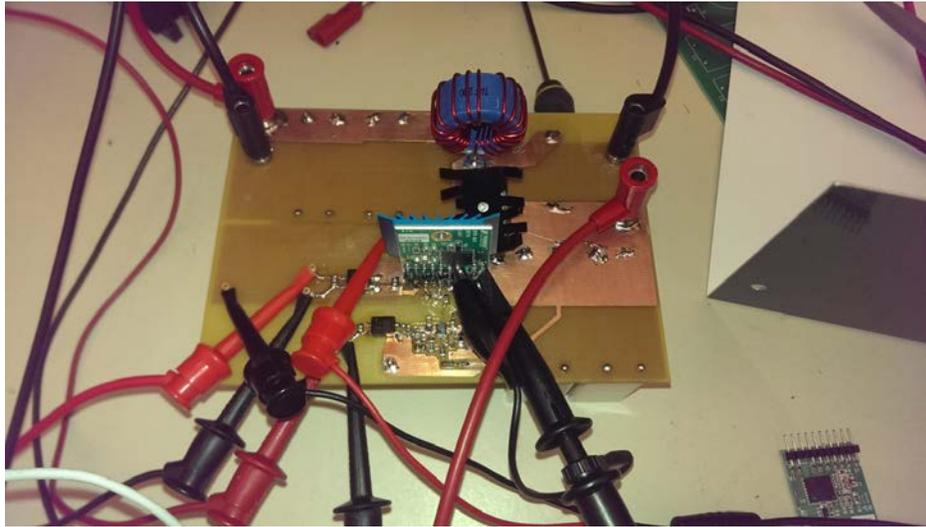
Figure 4. Non synchronous Boost Test Setup
