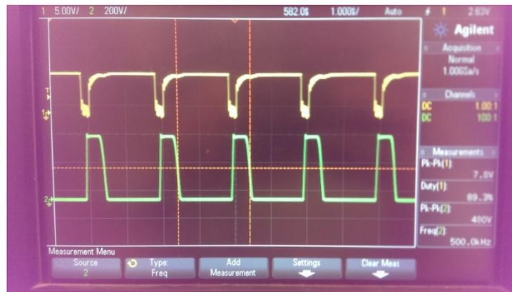
Figure 5. CH1 (yellow) Switch IN signal, CH2 (green) Drain to Source Voltage.  $V_{in}=100V$ ,  $V_{out}=480V$ .
