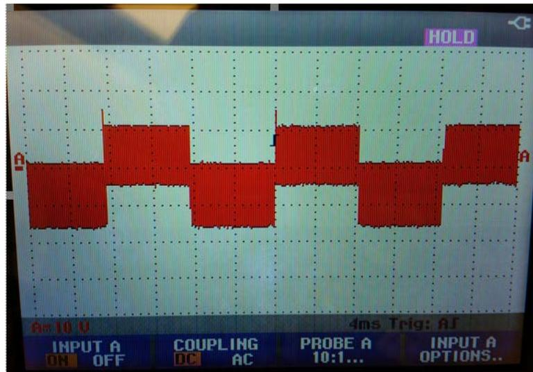
Figure 10. Inverter Stage Output
