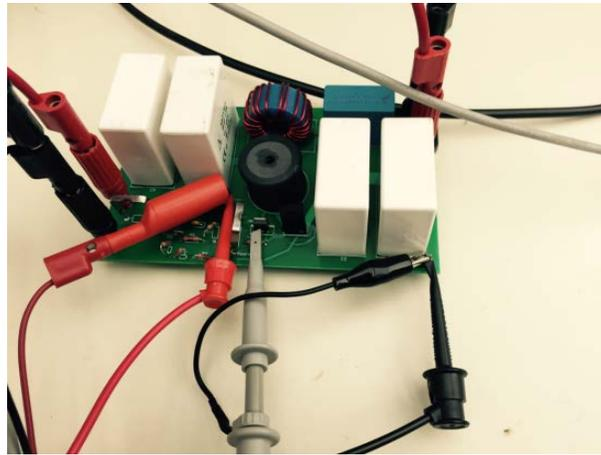
Figure 2. Input ripple suppressor boost circuit
