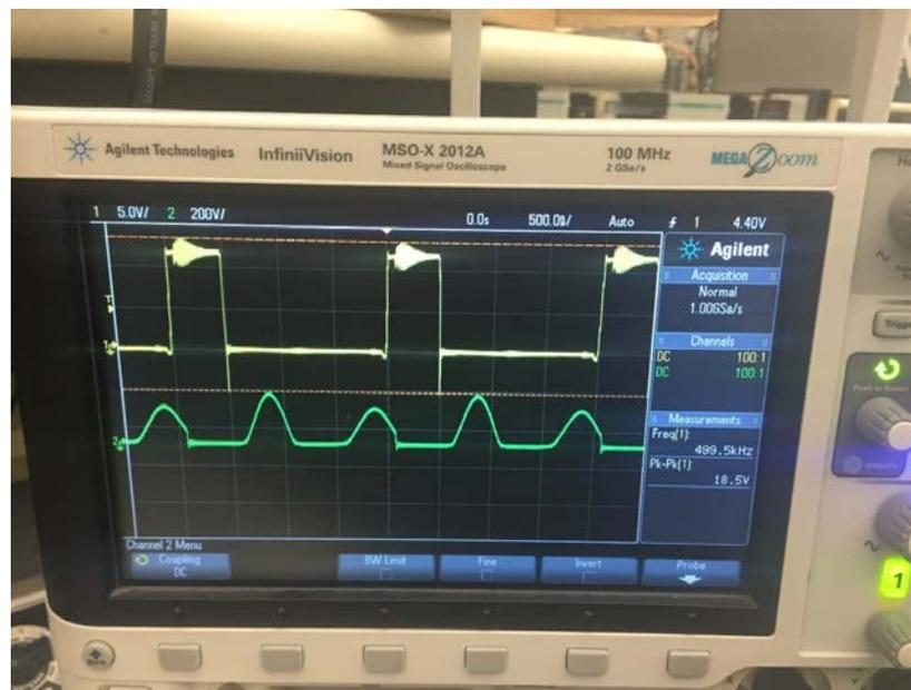
Figure 6. The Yellow waveform represents the Gate to Source Signal from the micro-controller
