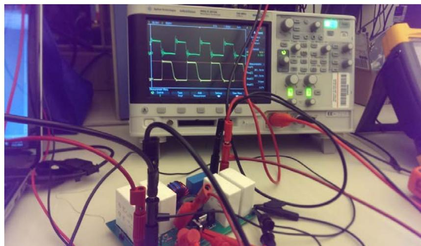
Figure 3. VGS (Green) and VDS (Yellow) waveforms with  $V_{in} = 40V$  and  $V_{out} = 500V$ .
