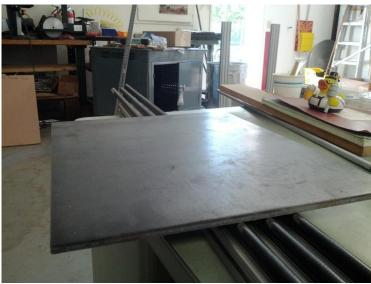
Figure 1: When connecting main tubes together, use a channel to keep the tubes straight while curing. This steel plates keeps the tubes seated in the channel while curing, ensuring a concentric tube connection.
