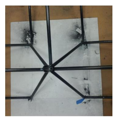
Figure 4: This is what the center section should begin to look like once three out of the four arms are in place. Note: At this state the connections are fragile and the airframe should not be handle or transported until additional tubes are bonded into place.
