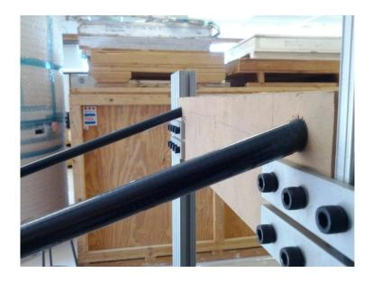
Figure 2: When cutting the main tubes to length prior to inserting into fixture, grind the ends down to match the angle of the end caps.
