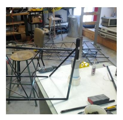
Figure 3: When constructing the center section, begin by cutting the center tube to length and setting in place on center. Then make each of the four downward angled tubes (you can see two in this photo connecting to the center tube ) and join them to the center.
