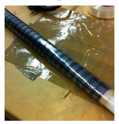
Figure 6: The 0-90 pre-preg with shrink tape applied.
