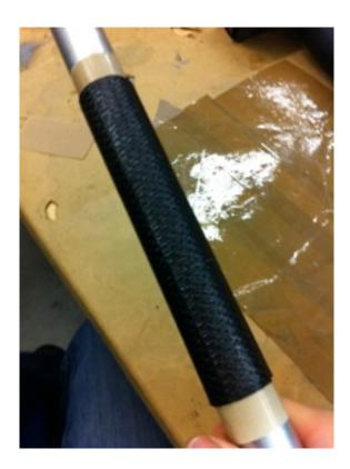
Figure 4: A steel mandrel with 4 layers of 0-90 pre-preg. It is ready for the shrink tape to be applied.
