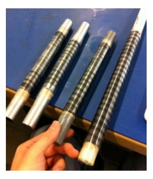
Figure 7: Two steel mandrels, a PVC mandrel and Polypropylene mandrels ready to be cured. The Polypropylene mandrel was easiest to remove from the carbon. The PVC mandrel did not handle the required heat well.
