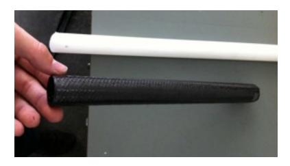
Figure 8b: A one foot 0-90 pre-preg spar after being removed from the mandrel.
