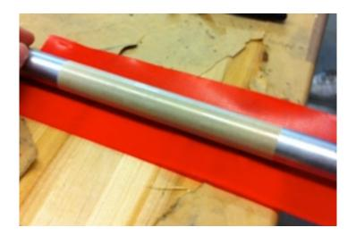
Figure 1: Wrapping the mandrel with teflon release cloth.
