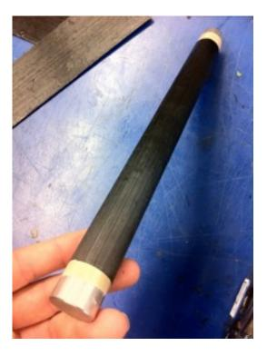
Figure 5: A steel mandrel showing the unidirectional layers ready for the shrink tape to be applied.
