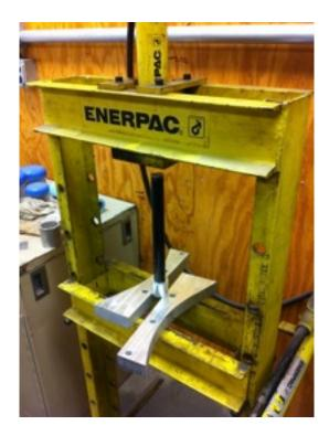
Figure 9: A hydraulic press being used to remove the mandrel from a unidirectional prepreg spar. I used a sleeve that was a net fit to the mandrel to shoulder against the carbon. The press is pushing the mandrel out the bottom.
