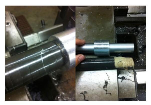
Figure 10: On one spar the teflon release cloth was adhered to the carbon by tape used to hold the cloth initially. The release cloth bunched up rather than coming out with the mandrel. Once it started to grow in thickness it split the end of the carbon tube and ruined the spar.
