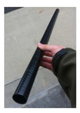
Figure 8a: A three foot unidirectional spar with 0,0,15,-15,0,0 layup after being removed from the polypropylene mandrel. I was able to pull it off the mandrel by hand. It weighed less than 8 ounces.
