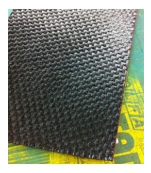
Figure 3: A closeup showing 0-90 pre-preg sheet. The 0-90 was only used for prototype tests due to the availability of the material. Unidirectional material was later used.
