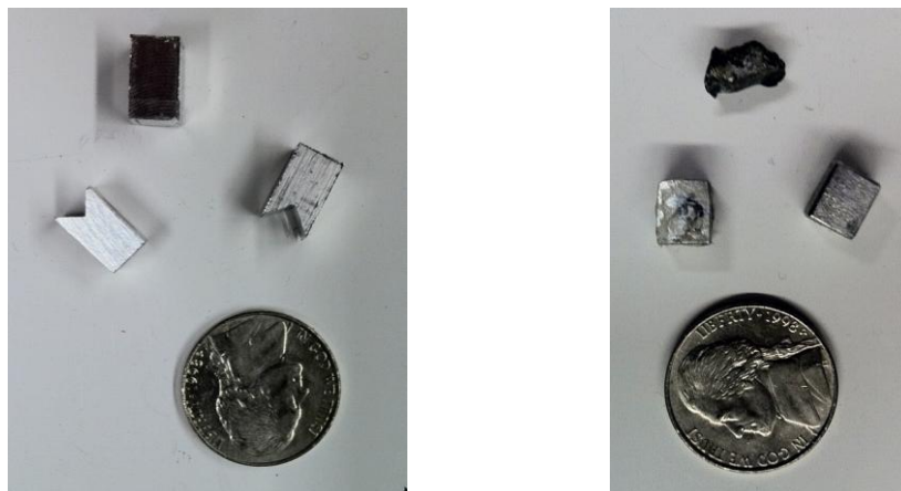
Figure 10 - Mk. 1 Projectiles Before (left) and After (right) firing
