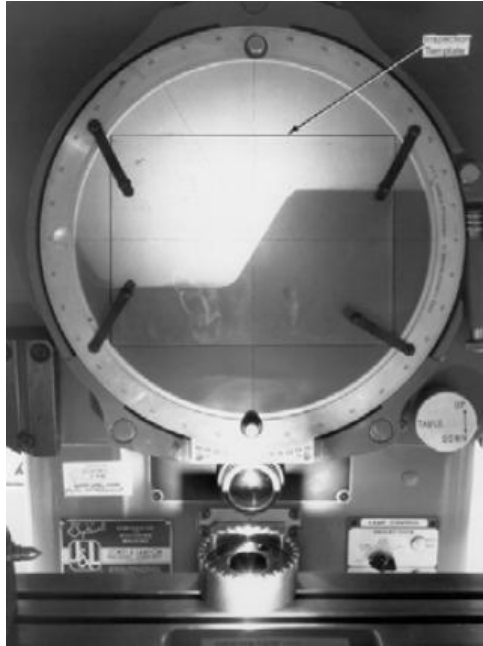
FIGURE 3. TOOTH FORM INSPECTION ON OPTICAL COMPARATOR, ADOPTED FROM [4]
