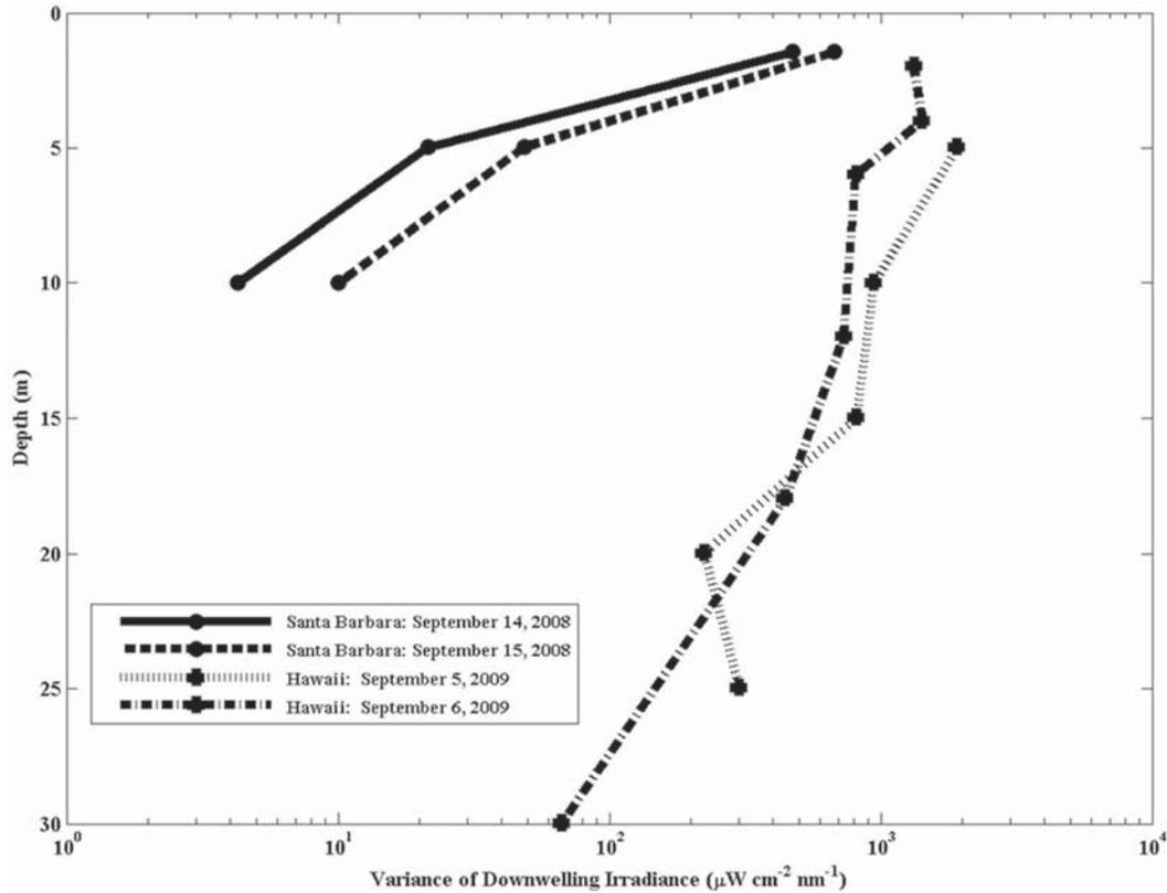
**Figure 10.** Variance in downwelling irradiance,  $E_d(\lambda)$ , measurements as a function of depth (m) made from the AUV for Santa Barbara Channel on 14 September and 15 September 2008 and off the Hawaiian Islands on 5 September and 6 September 2009.
