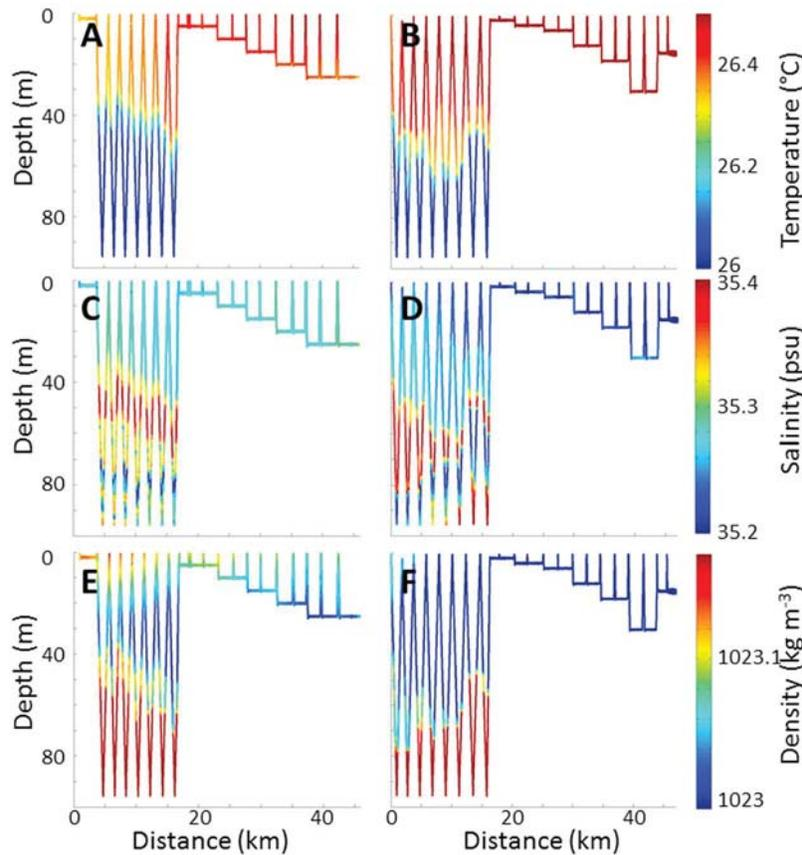
**Figure 4.** Depth distribution of temperature, salinity, and density as a function of distance measured by the REMUS AUV off the Hawaiian Islands (Figure 1c) on (a, c, e) 5 September and (b, d, f) 6 September 2009. The undulating patterns were in a “U” pattern starting on the northern edge.
