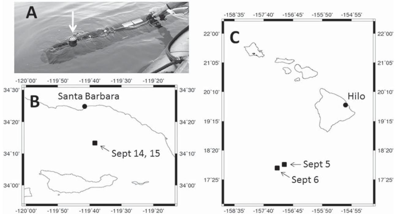
**Figure 1.** (a) REMUS autonomous underwater vehicle (AUV) with an integrated 7 wavelength radiometer for downwelling irradiance used in this study. Deployment sites for the AUV in (b) the Santa Barbara Channel on 14 and 15 September 2008 and (c) southwest of the island of Hawaii on 5 and 6 September 2009.
