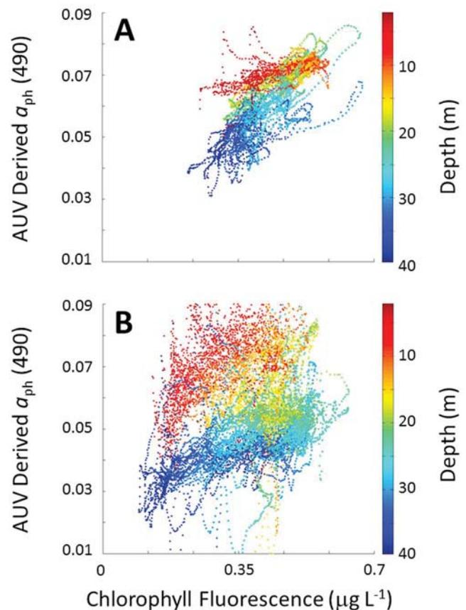
**Figure 9.** Relationship between derived phytoplankton absorption,  $a_{ph}$ , at 490 nm and measured chlorophyll *a* fluorescence ( $\mu\text{g L}^{-1}$ ) for Santa Barbara Channel on (a) 14 September and (b) 15 September 2008. Overlaid color represents the depths at which the measurements were made.
