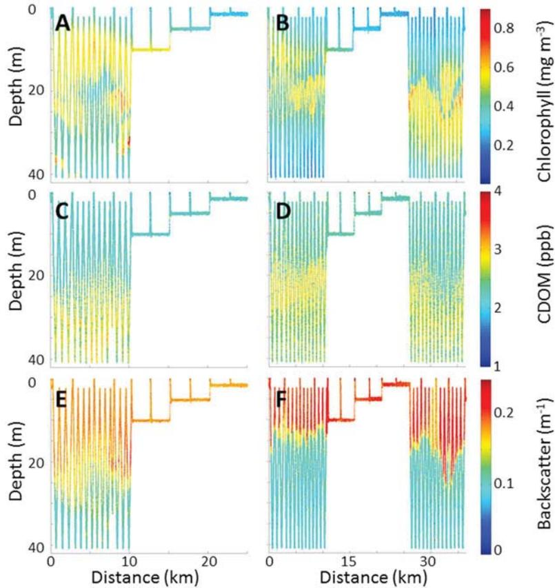
**Figure 3.** Depth distribution of chlorophyll *a*, CDOM and optical backscatter as a function of distance measured by the REMUS AUV for the Santa Barbara Channel on (a, c, e) 14 September and (b, d, f) 15 September 2008. Measurement patterns are identical to those in Figure 2.
