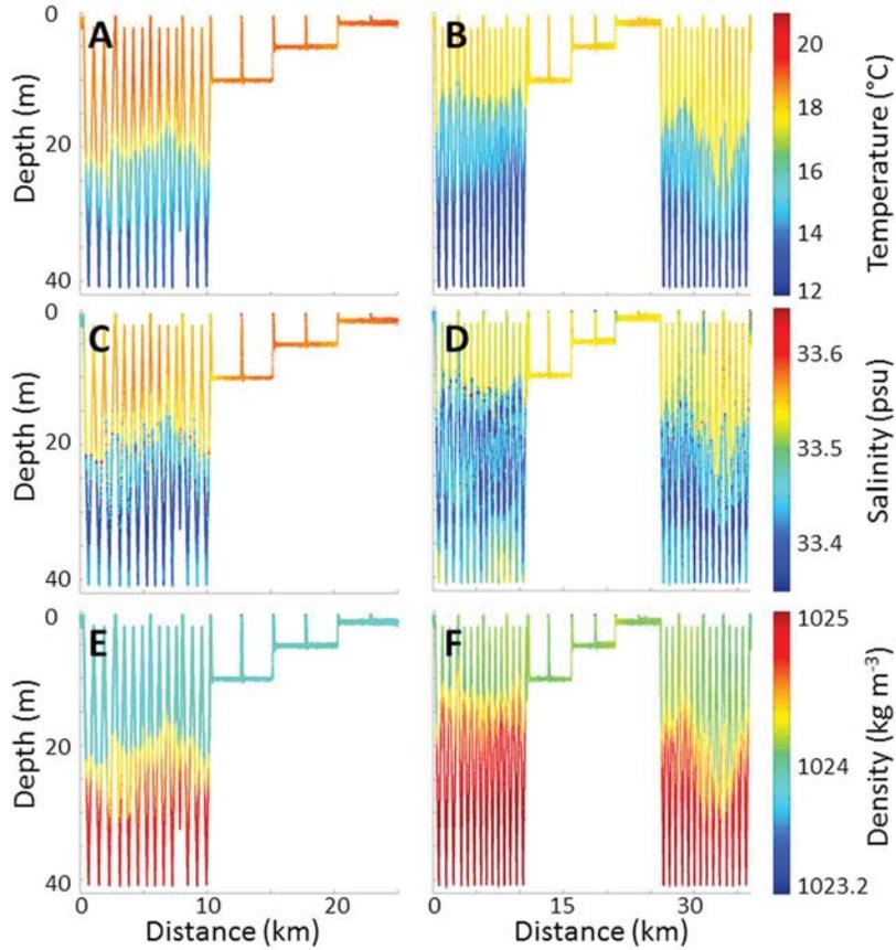
**Figure 2.** Depth distribution of temperature, salinity, and density as a function of distance measured by the REMUS AUV for the Santa Barbara Channel on (a, c, e) 14 September and (b, d, f) 15 September 2008. The undulating patterns were in a clockwise box pattern (Figure 1b) starting in the southeast corner. For 15 September 2008, the box was repeated.
