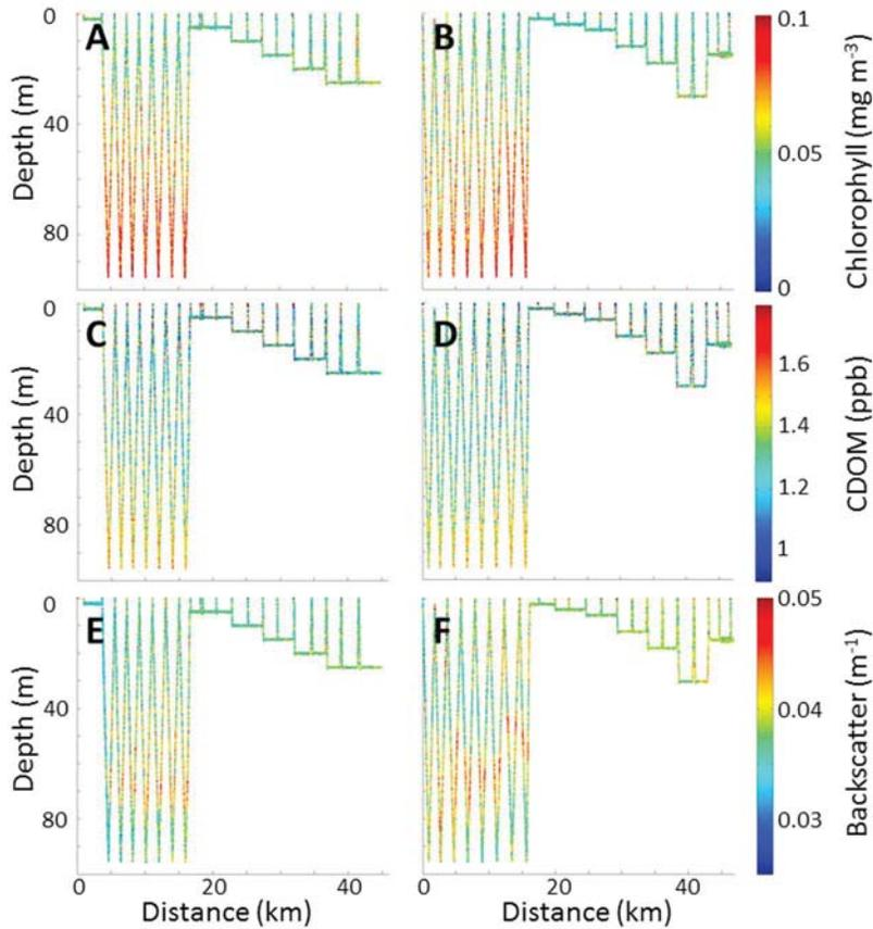
**Figure 5.** Depth distribution of chlorophyll *a*, CDOM and optical backscatter as a function of distance measured by the REMUS AUV off the Hawaiian Islands (Figure 1c) on (a, c, e) 5 September and (b, d, f) 6 September 2009. Measurement patterns are identical to those in Figure 4.
