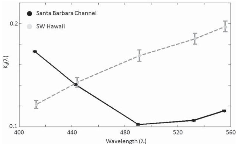
**Figure 6.** Mean spectral attenuation for data collected from the Santa Barbara Channel and the sampling station off the island of Hawaii. Means are shown with standard errors with wavelengths slightly offset for clarity.
