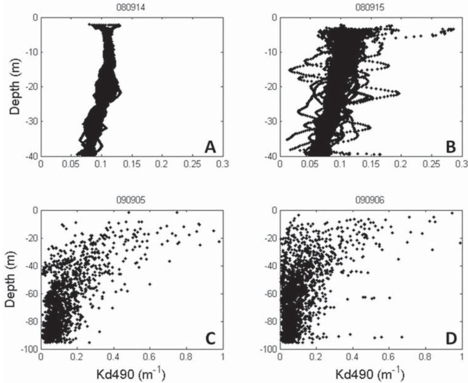
**Figure 7.** Downwelling attenuation coefficient at 490 nm,  $K_d(490)$ , as a function of depth (m) derived from AUV downwelling irradiance,  $E_d(\lambda)$ , measurements for Santa Barbara Channel on (a) 14 September and (b) 15 September 2008 and off the Hawaiian Islands on (c) 5 September and (d) 6 September 2009.
