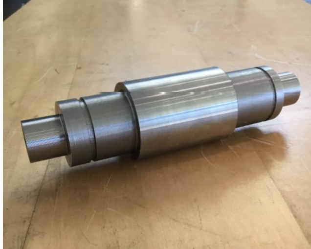
Figure 45. This is the intermediate shaft depicting the two grooves for the retaining rings. The intermediate shaft has two gears, thus the need for two retaining rings and their respective grooves.
