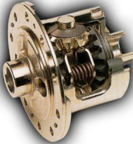
Figure 7. This Clutch Type LSD shows similarities with the open differential, but has an added spring between the side gears, and clutch discs between the side gears and housing [9].
