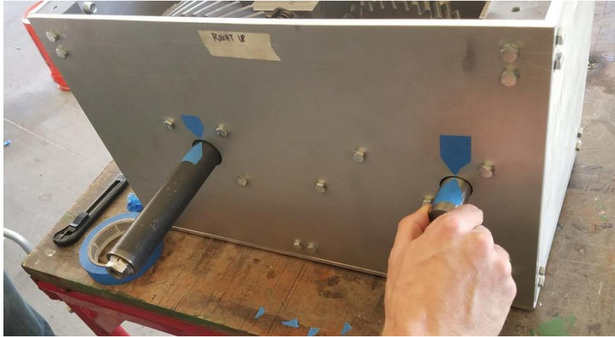
Figure 57. Our experimental setup was very simple and required very few additional supplies. The tape markers helped us keep track of the revolutions of each shaft.
