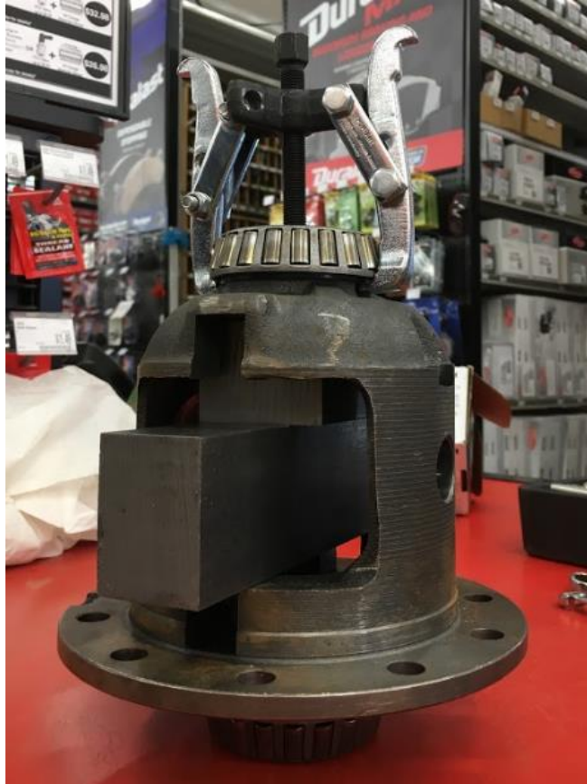
Figure 50. This bearing came off with the use of the bearing puller shown. The puller consists of the arms that have a lip to grab on the bottom of the bearing and a threaded rod to apply force to a stationary surface. We used steel blocks stacked inside the differential to provide a surface to apply force.
