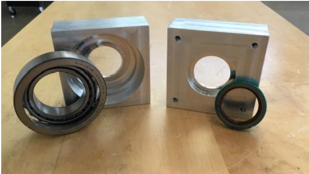
Figure 43. This bearing mount is one of the more complex designs due to having more features. A counterbore was required for the bearing as well as the seal for the input shaft.
