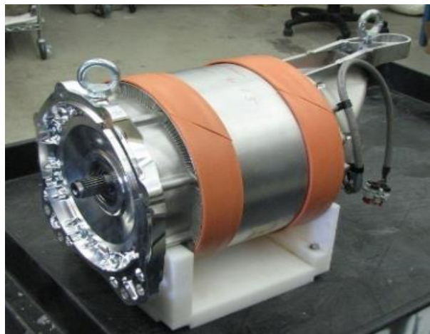
Figure 12: Motor-Drivetrain interface in a Tesla Model S [3]
