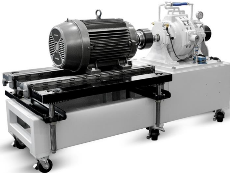
Figure 18. Electric motor on the left coupled to an absorption dynamometer on the right [19].
