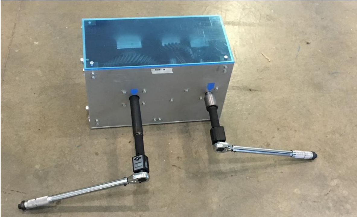
Figure 58. The input shaft with a torque wrench on the right-hand side is used to input the torque to the drivetrain. The corresponding output torque will read from the digital adapter coupled to the torque wrench on the left-hand side.
