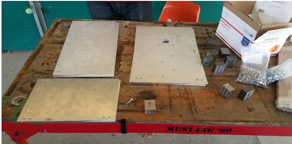
Figure 47. The CNC'ed housing plates with all of the necessary holes to bolts the housing together and the bearing mounts. The corner blocks and bolts needed to fasten the plates together are shown in the right of the picture.
