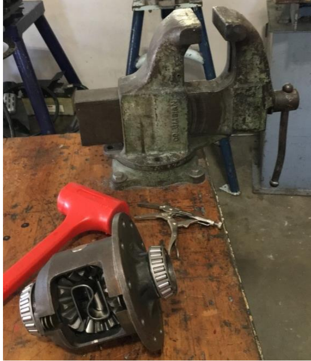
Figure 53. Tools required to install the S-spring include a vise, needle-nosed vise grips, and a mallet.
