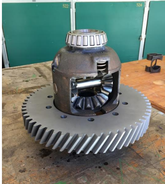
Figure 49. The holes drilled in the ring gear lined up perfectly with the holes on the flange of the differential. Not pictured here are the bolts used to mount the gear to differential itself.
