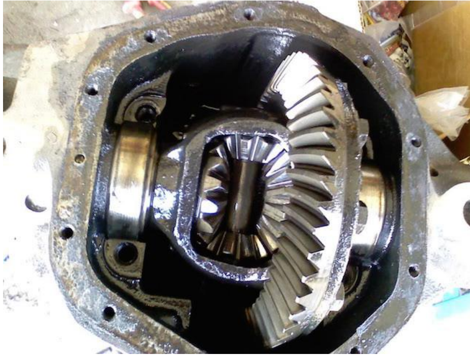
Figure 6. The layout of the gearing mechanisms used in open differentials [6].
