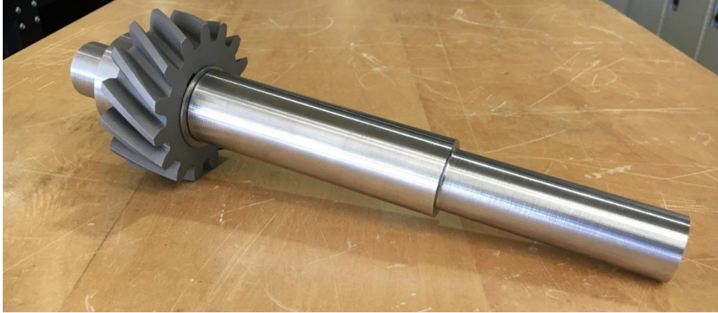
Figure 54. Above is the assembled input shaft with the retaining ring holding the pinion in place pressed up against the shoulder on the left-hand side. The key prevents the gear from freely spinning on the shaft when experiencing a torque.
