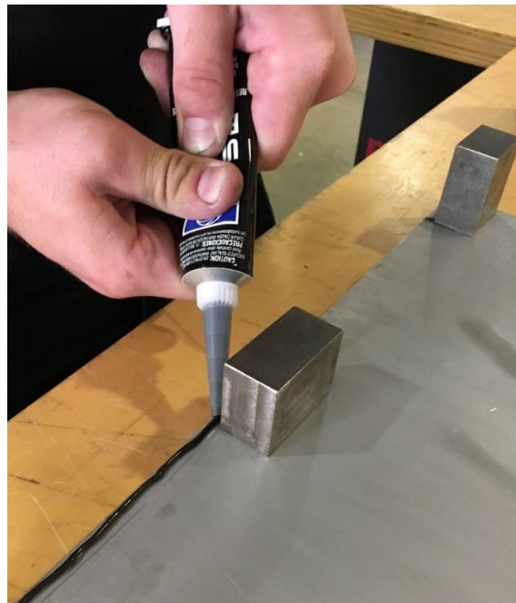
Figure 55. This how we applied RTV initially on the bottom plate. The left side plate was set directly on the line of RTV and bolted to the housing blocks.
