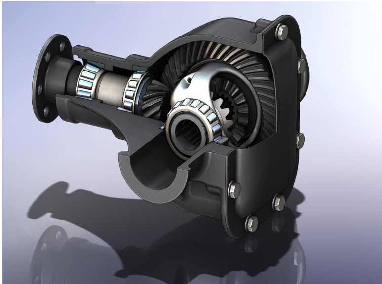
Figure 10. Vertical, transverse parting line as shown by the plate bolted on the back of the differential [12].
