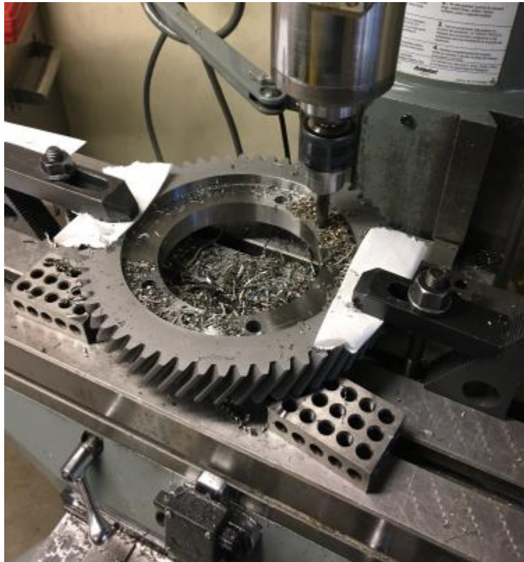
Figure 48. This is the fixturing used for drilling the holes in the ring gear. The 3-2-1 blocks raised the gear off the mill table to allow the drill to move all the way through without marking the table. The toe clamps held the gear in place.
