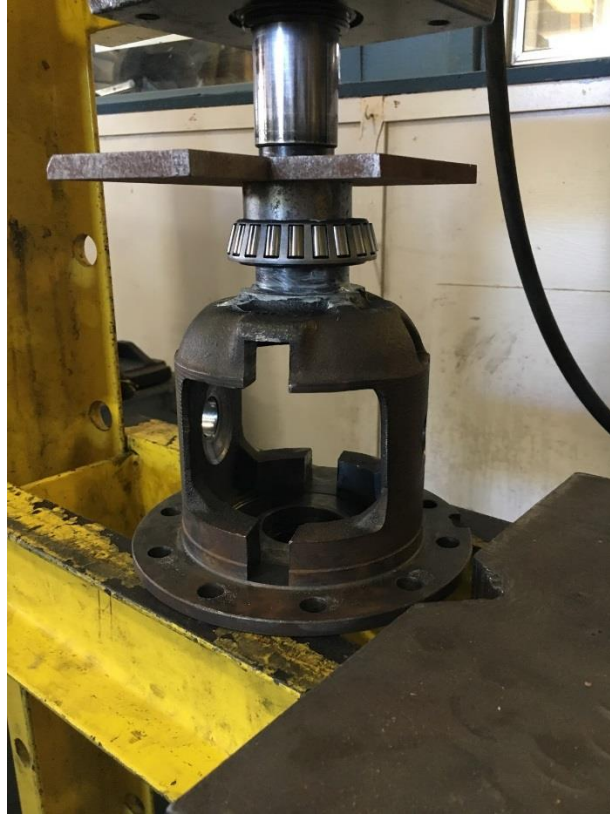
Figure 52. The hydraulic press with a small concentric tube to apply pressure to the inner race of the bearing without interfering with the differential. The plate on top is used to evenly apply pressure to the set up. We also greased the outer circular portion of the differential to allow the inner race of the bearing to slide on more easily.
