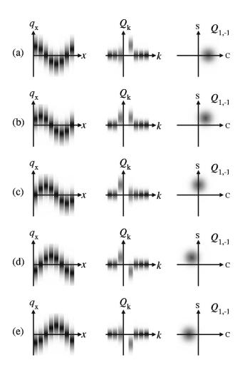
Fig. 18. Time evolution of the quantum mechanical lattice in a coherent, propagating |k|=1 state. This is a good visualization of a sound wave in a solid.
