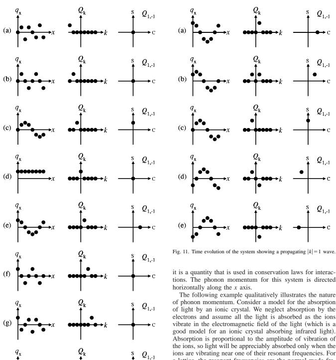
Fig. 10. All eight normal modes of the eight-particle lattice, from k = -3 in (a) to k=4 in (h), displayed using the coordinates used in Sec. III.
