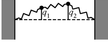
Fig. 1. A two-particle system, showing the position coordinates q_1 and q_2 of the two masses (dots), which are constrained to move vertically, connected by springs.
