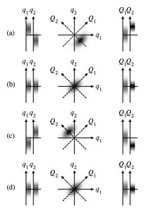
Fig. 6. Time evolution of a classical state of the two-particle system, shown at a different time scale than Fig. 5. In this eigenmode, the two masses oscillate against each other.
