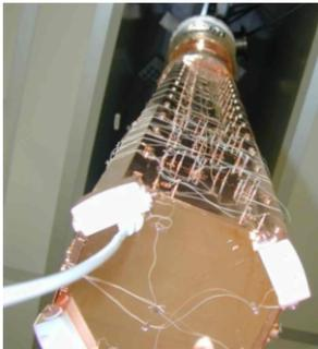
Figure 4. View of Cuoricino (from bottom) during installation.
