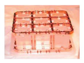
FIG. 1. (Color online) The Tower of CUORICINO and individual 4 and 9 detector modules.
