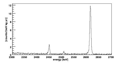
FIG. 5. The summed background spectrum in the  $\sim\!400~{\rm keV}$  region of interest, which includes the  $0~\nu\beta\beta$ -decay energy 2530.3  $\pm$  2.0 keV.
