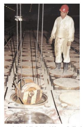
Figure 5.3. A crane at the Mayak Fissile Material Storage Facility, lowering fissile material into a 'nest'
