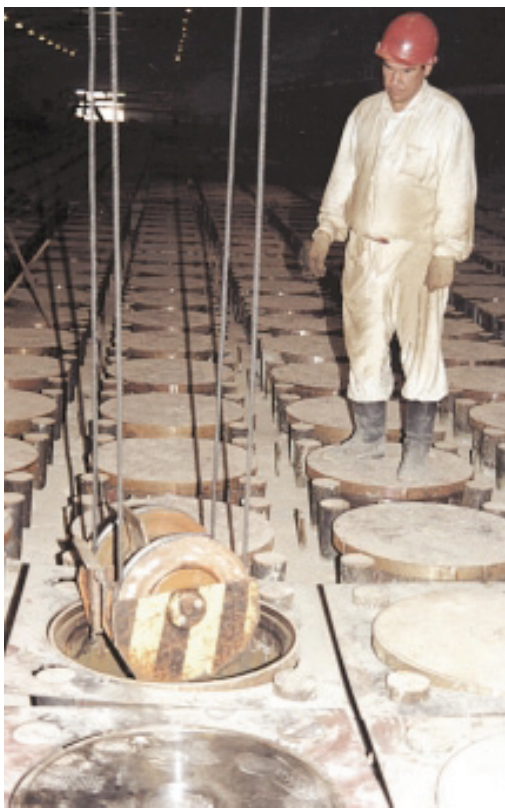
Figure 5.3. A crane at the Mayak Fissile Material Storage Facility, lowering fissile material into a ‘nest’
