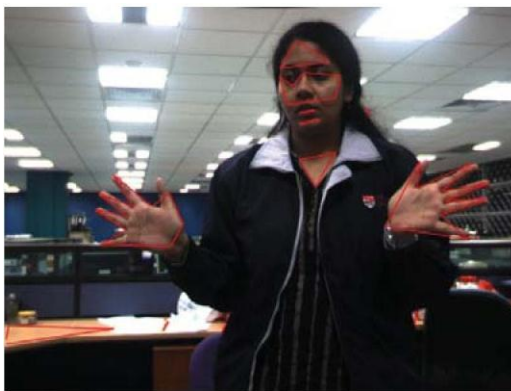
Figure 5: Douglas-Peucker Approximation - Shows the results of Douglas-Peucker approximation of the contours of the skin colored region.
