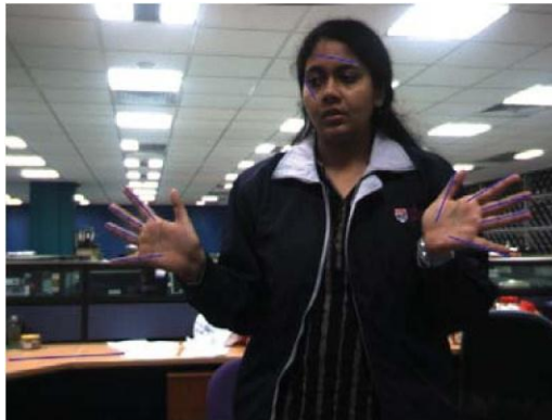
Figure 7: Results of using Finger Line Approximation Algorithm - Shows the result of running the line approximation algorithm on the approximated contour shown in previous figure. The lines found are drawn in blue.
