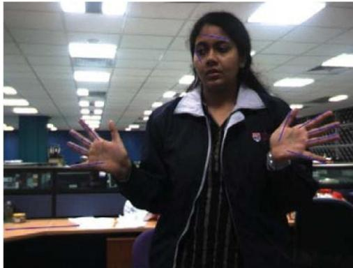
Figure 7: Results of using Finger Line Approximation Algorithm - Shows the result of running the line approximation algorithm on the approximated contour shown in previous figure. The lines found are drawn in blue.
