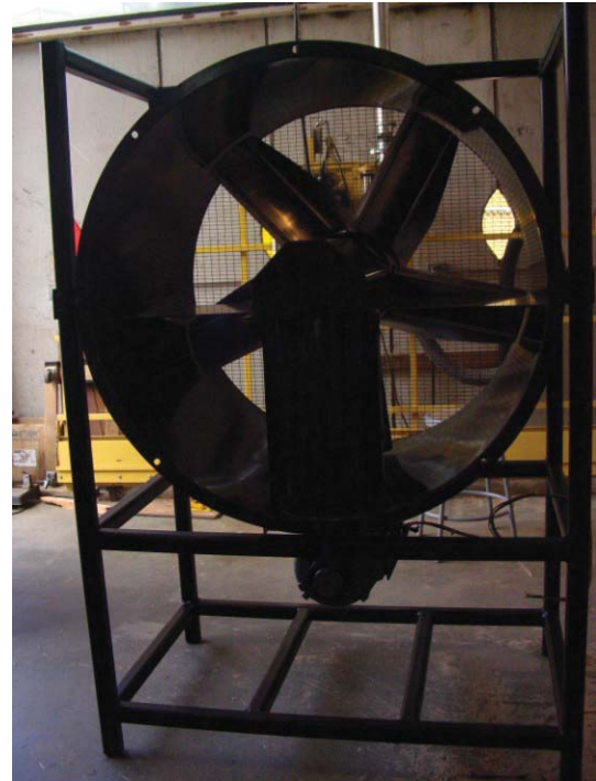
Figure 9. Completed nstallation of fan in motor stans
