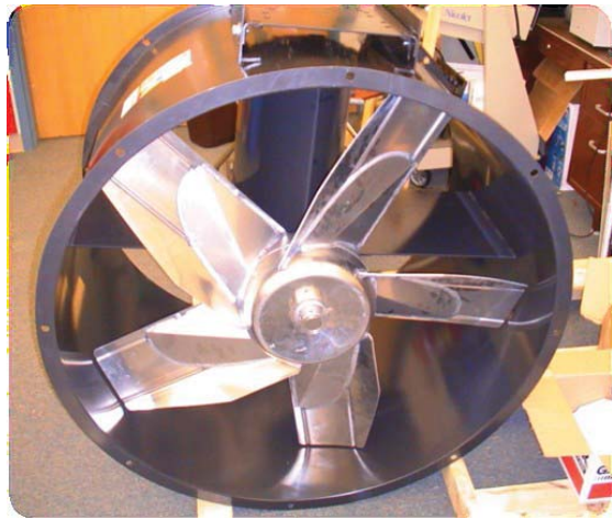
Figure 1. Dayton 42" Diameter, Belt Driven, Tube Axial Duct Fan. With 5hp motor capable of 25,320 CFM.
