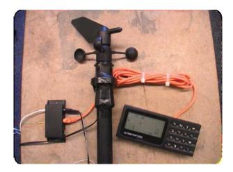
Figure 15. Anemometer and Ultimeter 2000.
