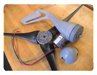
Figure 4. SunForce 400W Wind Generator. Peak output achieved at 28mph wind speed.
