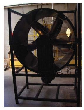
Figure 9. Completed nstallation of fan in motor stans
