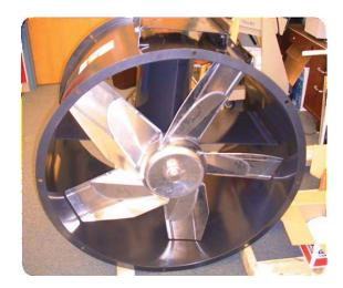
Figure 1. Dayton 42" Diameter, Belt Driven, Tube Axial Duct Fan. With 5hp motor capable of 25,320 CFM.
