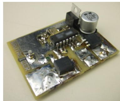
Figure 7. Transformer test circuit for Experiment #4
