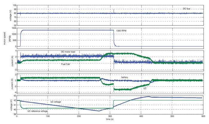
Fig. 6 Experimental results for an ideal start-stop cycle
