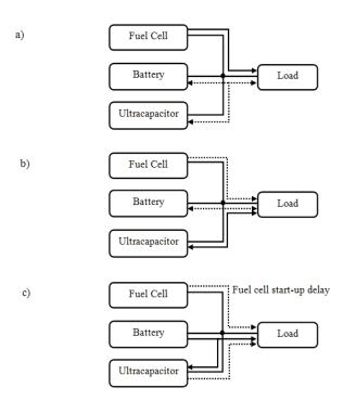
Fig. 1 Mode of power flow in the proposed hybrid system: a) during steady state, b) during transient, c) during start-up (solid arrow indicates of main power flow, dotted arrow indicates of secondary power flow)
