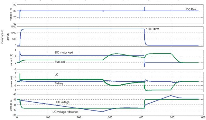
Fig. 5 Simulation results for an ideal start-stop cycle
