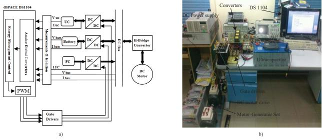
Fig. 4 Proposed implementation (a) Block diagram of the experimental set-up (b) Picture of complete experimental set-up
