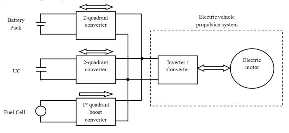
Fig. 2 Proposed parallel energy sharing system
