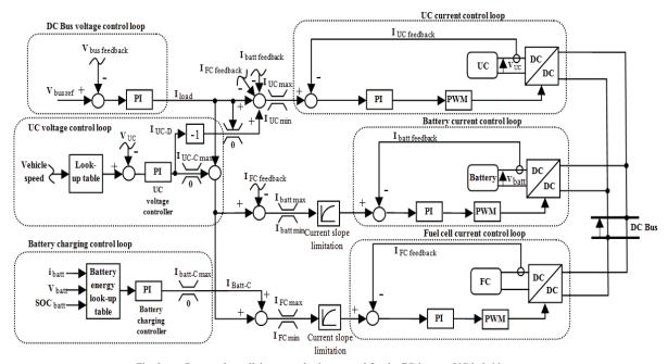
Fig. 3 Proposed parallel energy-sharing control for the FC-battery-UC hybrid system
