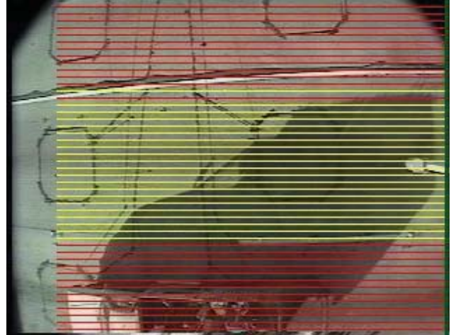
Figure 6. Shadow rejection method illustrated in diagnostic mode. Detection scan lines in lane do not terminate on leading edge of shadow, indicating rejection of shadow flow front.
