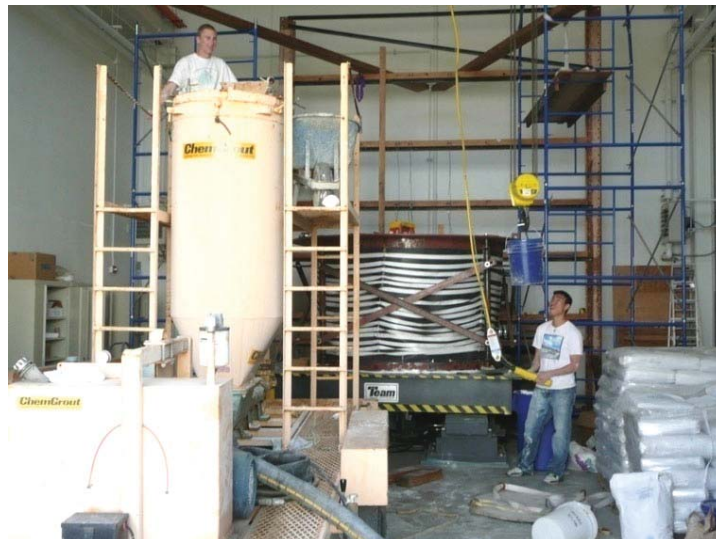
Figure 7. The flexible wall barrel is composed of the four corner posts with universal joints at the top and bottom, the top and bottom rings, and the barrel wall. The wall is composed of a 6.4 mm thick rubber membrane which is confined by 45 mm wide Kevlar straps spaced on center every 60 mm. The (yellow) mixer on the left is used to mix the large volumes of model soil (composed of kaolinite, bentonite, fly ash, and water) for filling the barrel.
