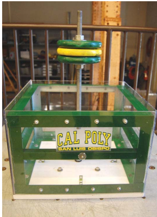
Figure 8. During phase one, the natural frequency of various SDOF setups are determined using the small shake table. The foundation is 46cm by 46cm, and the “ basement ” walls are 32cm tall.
