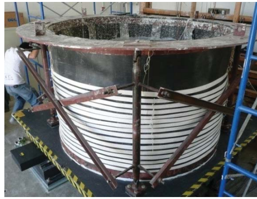
Figure 4. The testing platform shown consists of the shake table and flexible wall barrel at Cal Poly's Parsons Earthquake Lab.
