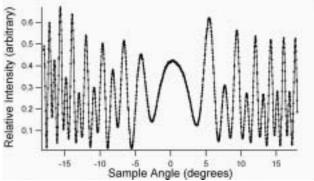
Figure 1. Observed data of the interferometric fringe pattern intensity as a function of the sample angle, for the ZnGeP<sub>2</sub> sample.
