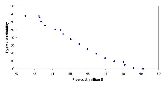
Figure 3. Pareto optimal solutions of pipe cost and hydraulic reliability
