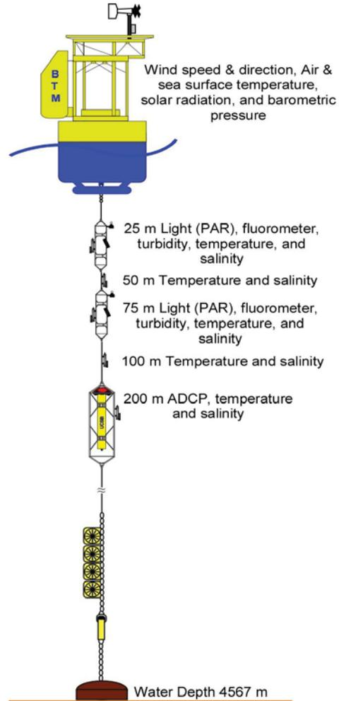
**Figure 2: Schematic diagram of the Bermuda Testbed Mooring - a deep-sea mooring that produces 302,800 Bpd**
