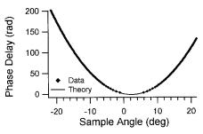
Fig. 4. Experimental and calculated angular phase delay for the interferogram of Fig. 3 as a function of the incident angle,  $\theta$ .
