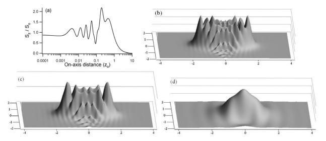
Fig. 4. Calculated intensity of the normalized z-component of the Poynting vector (a) as a function of axial distance from the aperture plane, and beam profiles for (b) an axial distance of  $z_1 = 0.054$ , (c)  $z_1 = 0.09$ , and (d)  $z_1 = 0.46$ , where  $z_1$  is the on-axis distance normalized to  $z_0 = ka^2$ .
