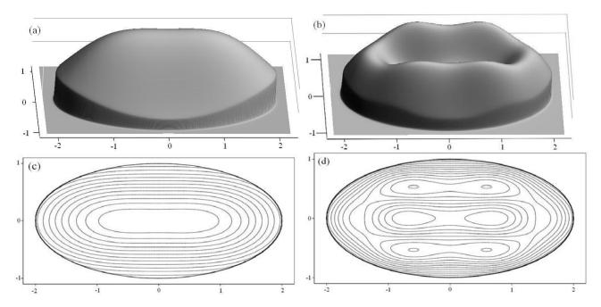
Fig. 1. Intensity distributions of the normalized z-component of the Poynting vector in the aperture plane for (a)  $a = \lambda/2$  and  $b = \lambda$ , (b)  $a = \lambda$  and  $b = 2\lambda$ , and their corresponding contour plots, (c) and (d), respectively, where a is the minor axis, b is the major axis, and the polarization of the incident light is aligned with the major axis.
