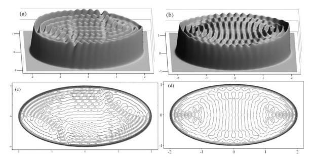
Fig. 3. Intensity distributions of the normalized z-component of the Poynting vector in the aperture plane for  $a = 5\lambda$  and  $b = 10\lambda$ , with the incident polarization at an angle of (a)  $\pi/4$  with respect to the major axis, (b) aligned with the minor axis, and their corresponding contour plots, (c) and (d), respectively.
