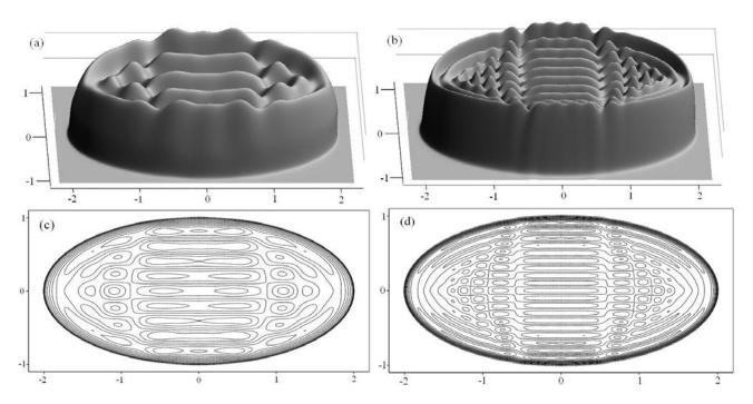
Fig. 2. Intensity distributions of the normalized z-component of the Poynting vector in the aperture plane for (a)  $a = 2.5\lambda$  and  $b = 5\lambda$ , (b)  $a = 5\lambda$  and  $b = 10\lambda$ , and their corresponding contour plots, (c) and (d), respectively, where a is the minor axis, b is the major axis, and the polarization of the incident light is aligned with the major axis.
