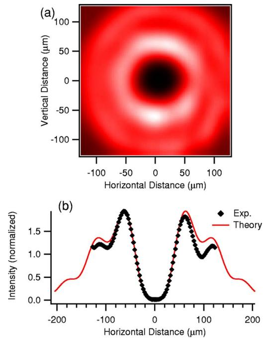
FIG. 6. (Color online) (a) Experimental scan of the beam profile for  $\lambda = 10.61 \mu\text{m}$ ,  $a = 205 \mu\text{m}$ ,  $z = 2 \text{ mm}$ , and (b) the radial beam profile versus Hertz vector diffraction theory.
