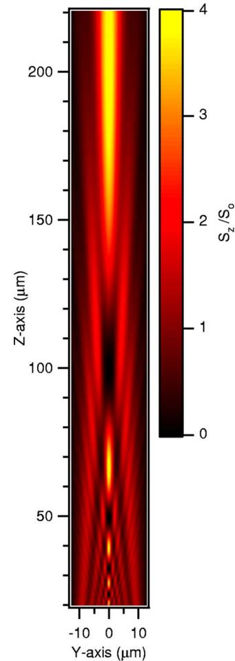
FIG. 1. (Color online) Calculated color image plot of the  $z$  component of the Poynting vector versus  $y$  and  $z$  for plane-wave,  $x$ -polarized, 780-nm light incident upon a 25- $\mu\text{m}$  aperture. The relative intensity is normalized to the intensity incident upon the aperture.
