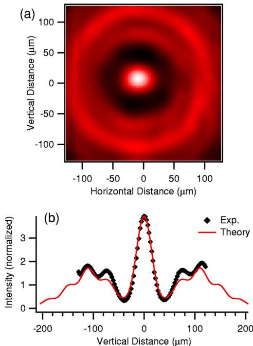
FIG. 5. (Color online) (a) Experimental scan of the beam profile for  $\lambda = 10.61 \mu\text{m}$ ,  $a = 205 \mu\text{m}$ ,  $z = 1.33 \text{ mm}$ , and (b) the radial beam profile versus Hertz vector diffraction theory.
