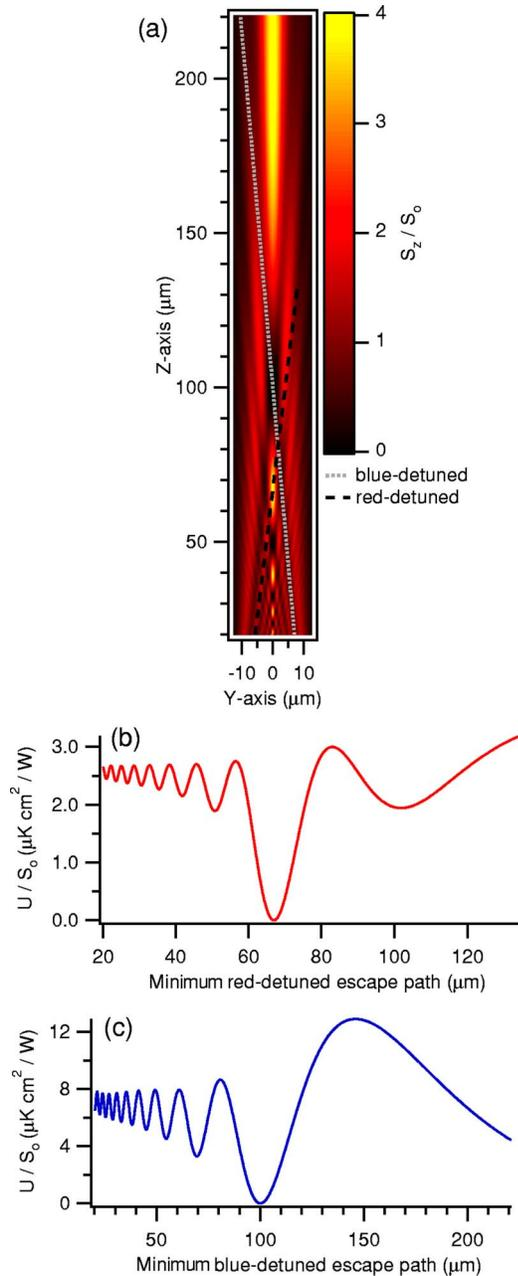
FIG. 3. (Color online) (a) Illustration of the minimum escape path from the on-axis dipole trap for red- and blue-detuned laser light. (b) and (c) are the dipole trap depths (in  $\mu\text{K}$  per  $\text{W}/\text{cm}^2$  of laser intensity incident upon the aperture) for  $^{85}\text{Rb}$  with  $\Delta = -10^4\Gamma$  and  $\Delta = 10^3\Gamma$  versus position along the red- and blue-detuned minimum escape paths, respectively.
