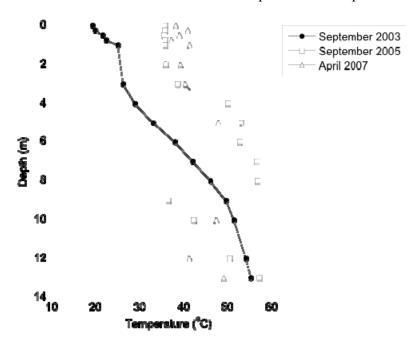
Figure 3. Variation of waste temperatures due to overfilling.
