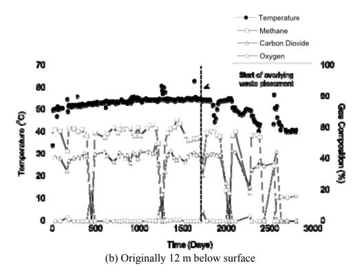
Figure 2. Temperature-gas relationships in MSW landfills due to overfilling.
