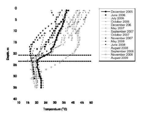
Figure 4. Variation of waste temperatures under semi-aerobic conditions.
