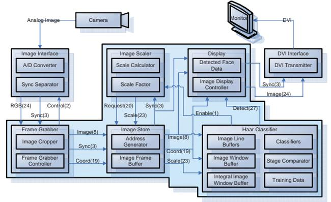
Figure 5. Block diagram of proposed face detection system.
