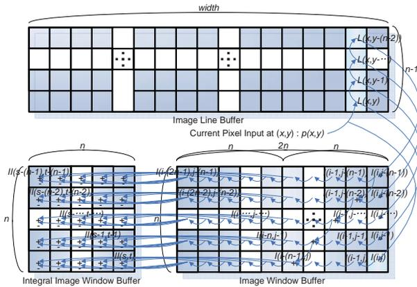
Figure 7. Architecture for generating integral image window.
