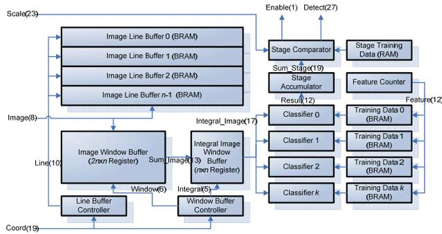
Figure 6. Block diagram of proposed face detection system.
