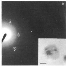
Fe<sub>3</sub>O<sub>4</sub> and Fe<sub>3</sub>S<sub>4</sub> in a bacterium
