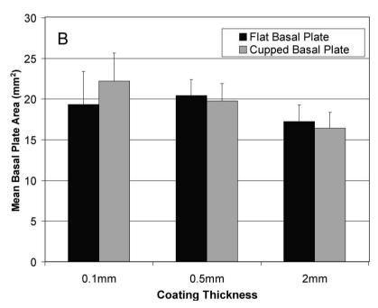
Figure 4. Mean area of the basal plates of barnacles grown on three thicknesses of PDMS, as measured during shear testing. A = mean area for all barnacles on each of three thicknesses; B = mean area of barnacles exhibiting the typical ("flat") basal plate and the atypical ("cupped") basal plate.
